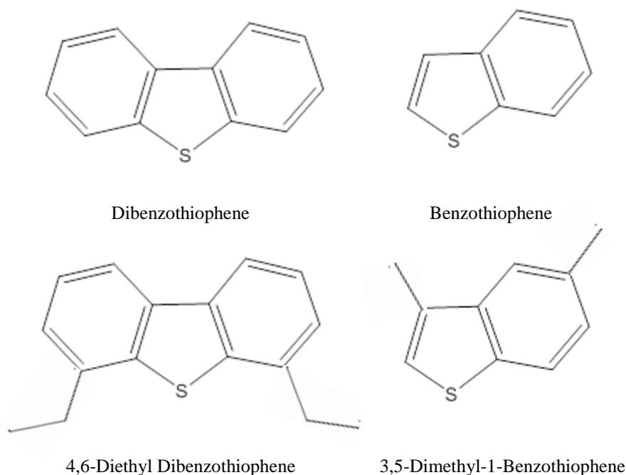
**Figure 2-1** Dibenzothiophene (DBT), benzothiophene (BT) and an alkylated derivative of each
