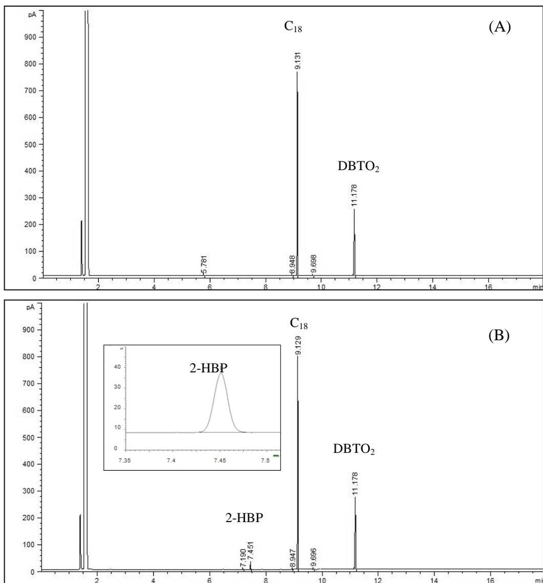
**Figure 4-6** Comparison of Gas Chromatograms for *R. rhodochrous* IGTS8 grown in SFMM with 1.0mM DBTO<sub>2</sub>. Samples were taken at time zero (A) and after 48 hours (B) of incubation
