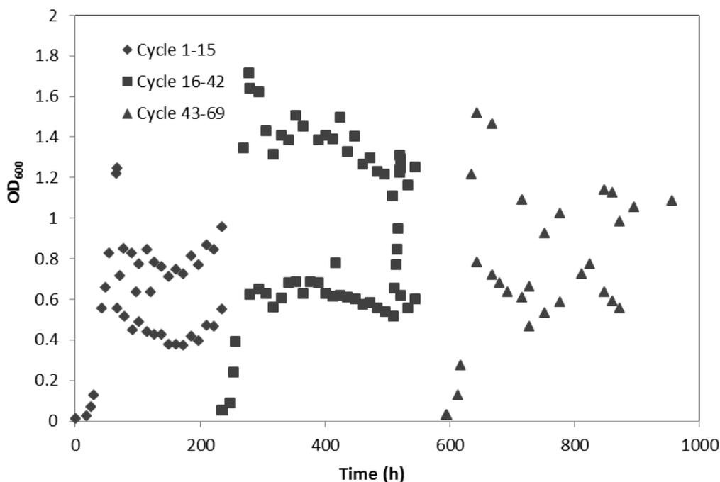
**Figure 4-24** Optical density measurements during SCF operation of *R. rhodochrous* IGTS8 for 69 cycles in SFMM with 0.25mM DBTO<sub>2</sub> and 14mM DMFA
