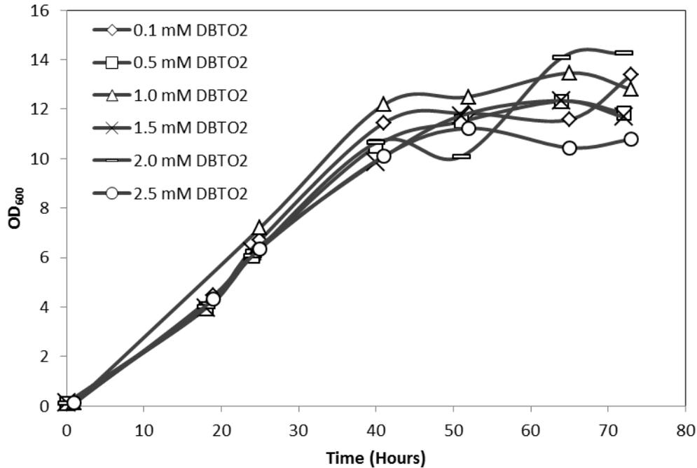
**Figure 4-2** Optical density measurements for cultures of *R. K1bD* growing in TSB with varying concentrations of DBTO<sub>2</sub> (◇ 0mM, △ 0.1mM, × 0.5mM, \*1.0mM, ○ 1.5mM, □ 2.0mM, and – 2.5mM)
