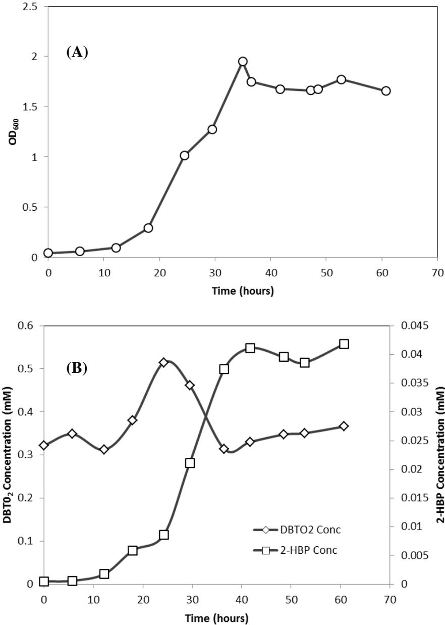
**Figure 4-8** (A) Optical density values and (B) concentration of DBTO<sub>2</sub> (◇) and 2-HBP in cultures of *R. rhodochrous* IGTS8 grown in SFMM with 0.5mM DBTO<sub>2</sub>
