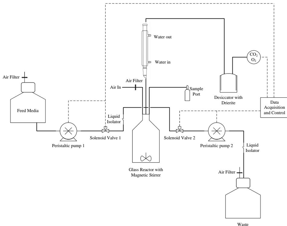
**Figure 3-1** Schematic of the Self-Cycling Fermentation (SCF) system
