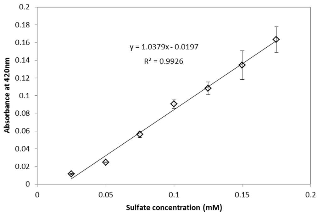
**Figure 3-4** Calibration curve for absorbance at 420nm for varying concentrations of sulfate
