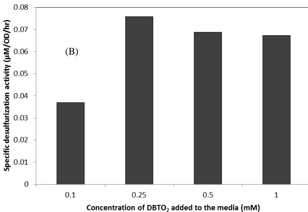
**Figure 4-10** Comparison of growth (A) and specific desulfurization activity (B) for *R. rhodochrous* IGTS8 in SFMM with varying concentrations of DBTO<sub>2</sub> (0.1mM (×), 0.25mM (\*), 0.5mM (o) and 1.0mM (◇))
