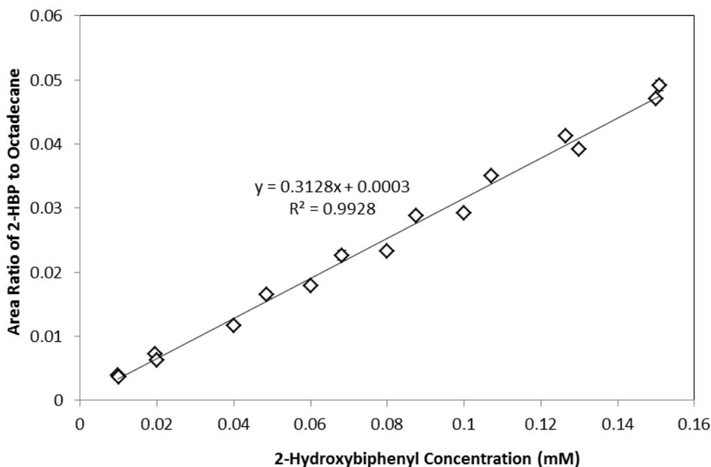
**Figure 3-2** Gas chromatography calibration curve for 2-HBP with octadecane as an internal standard
