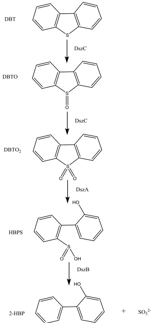
**Figure 2-3** 4S pathway for the desulfurization of DBT (adapted from Soleimani et al. (2007))
