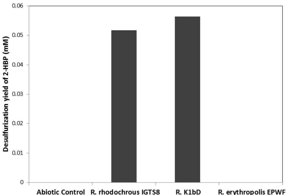
**Figure 4-12** Desulfurization yield of 2-HBP after 48 hours in cultures of *R. rhodochrous* IGTS8, *R. K1bD*, and *R. erythropolis* EPWF grown in SFMM with 0.25mM DBTO<sub>2</sub> and 14mM DMFA. An abiotic control is included for comparison
