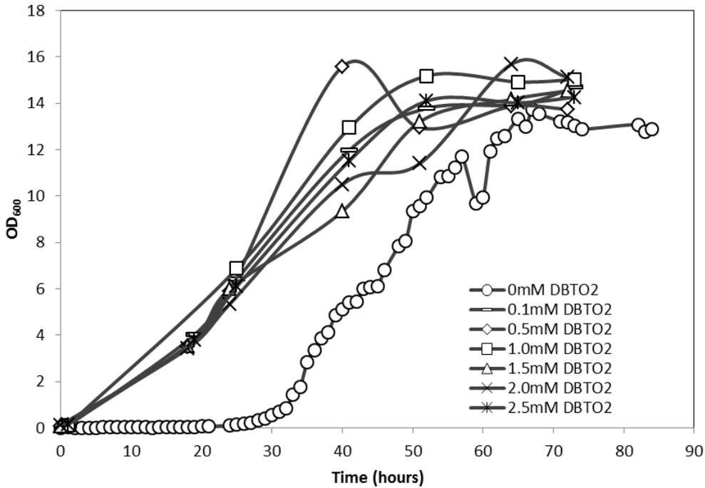
**Figure 4-3** Optical density measurements for cultures of *R. erythropolis* EPWF growing in TSB with varying concentrations of DBTO<sub>2</sub> (○ 0mM, — 0.1mM, ◇ 0.5mM, □ 1.0mM, △ 1.5mM, x 2.0mM, and \* 2.5mM)
