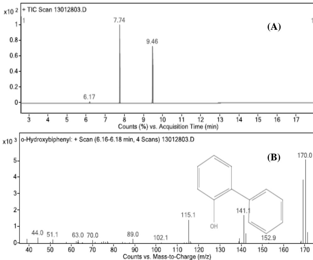
**Figure 4-7 (A)** Chromatogram from the gas chromatography-mass spectrometry analysis and **(B)** identification of 2-HBP by gas chromatography -mass spectrometry for *R. rhodochrous* IGTS8 in SFMM with 1.0mM DBTO<sub>2</sub> at 48 hours
