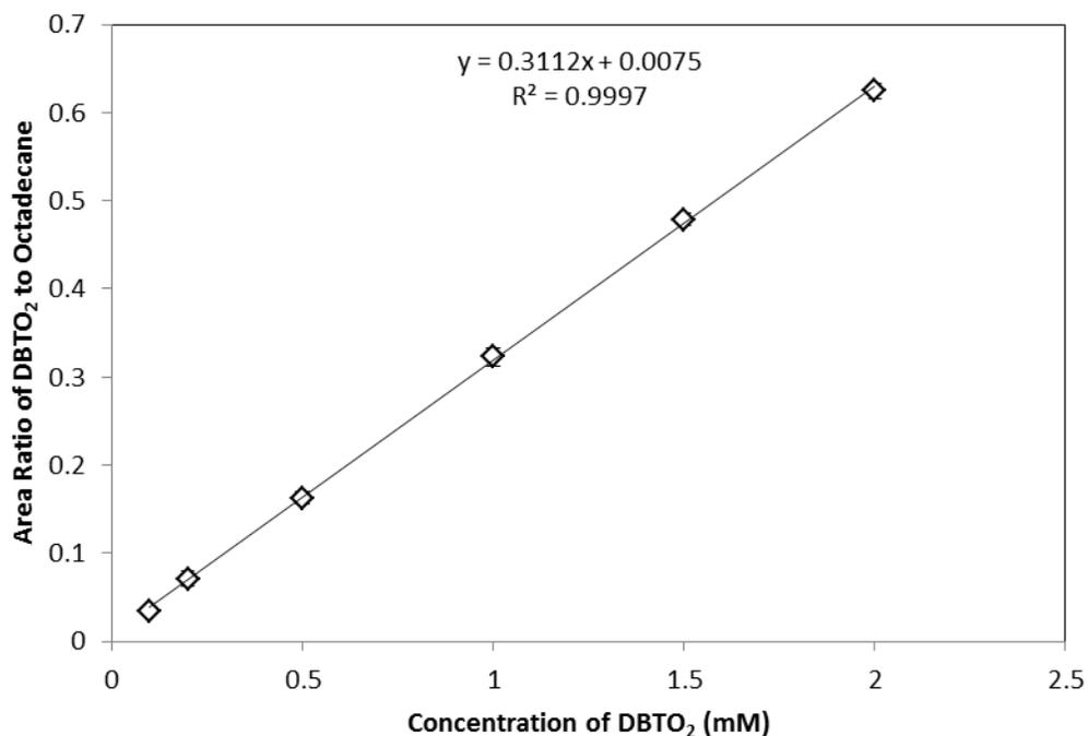
**Figure 3-3** Gas chromatography calibration curve for DBTO<sub>2</sub> with octadecane as an internal standard
