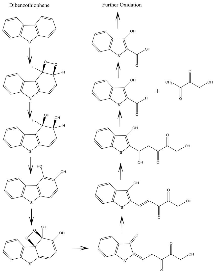
**Figure 2-2** Kodama pathway for the biodesulfurization of dibenzothiophene (DBT) (figure adapted from Soleimani et al. (2007))
