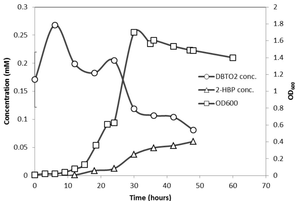
**Figure 4-9** DBTO<sub>2</sub> concentration (O), 2-HBP concentration (Δ), and optical density values at 600nm (□) for *R. rhodochrous* IGTS8 grown in SFMM with 0.25mM DBTO<sub>2</sub> and 14mM DMFA
