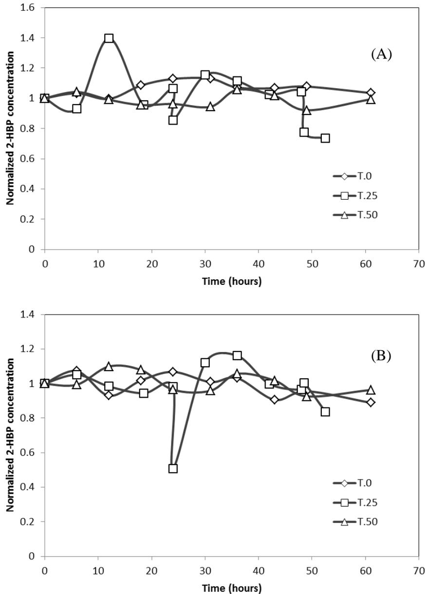
**Figure 4-15** Normalized values of 2-HBP concentration for *R. rhodochrous* IGTS8 original inoculum ( $\diamond$ ), T.25 ( $\square$ ) and T.50 ( $\triangle$ ) (transferred in SFMM + 1.0mM DBTO<sub>2</sub>) grown in SFMM with 2-HBP (A) in MSM with 2-HBP (B)
