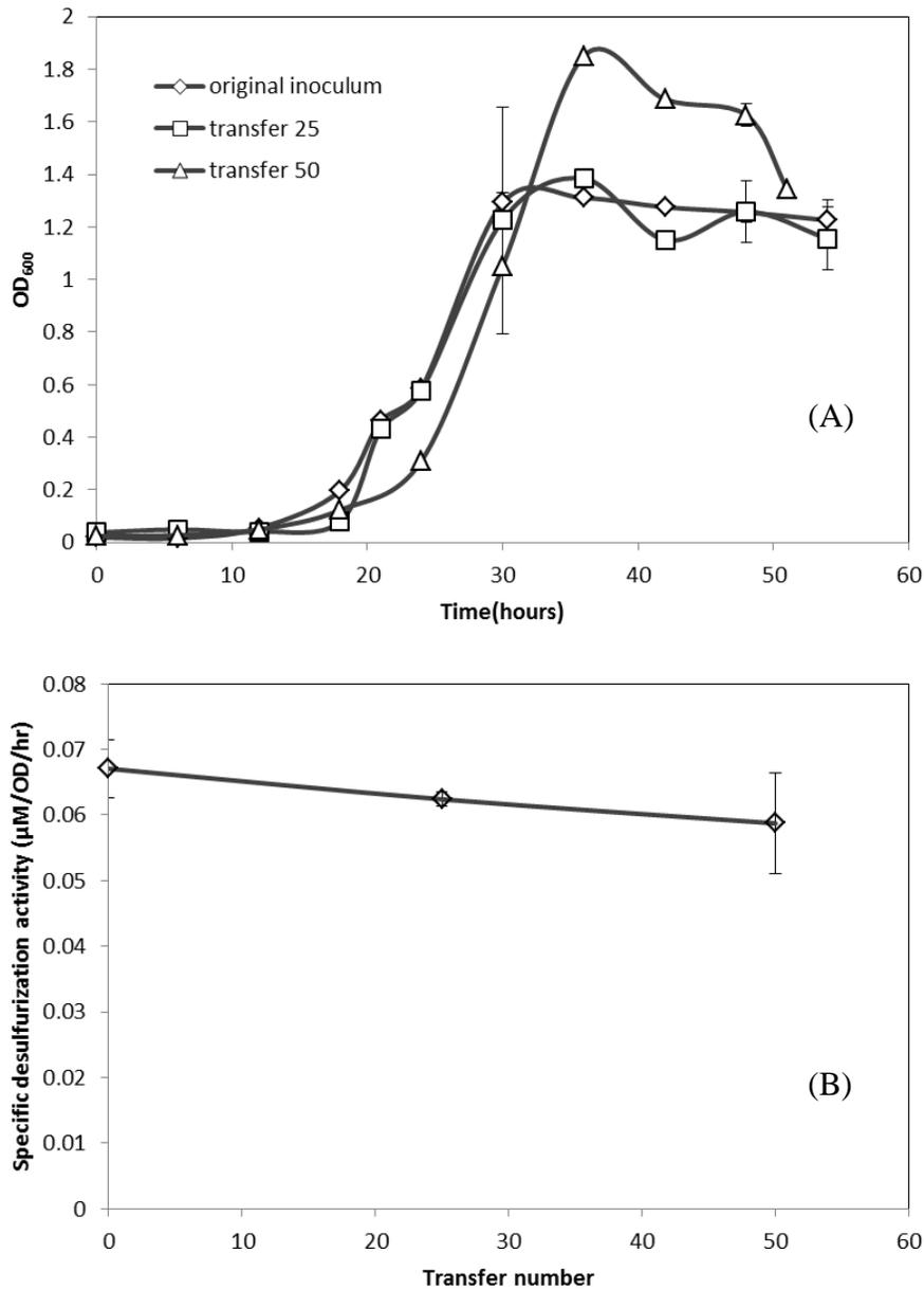
**Figure 4-23** Comparison of growth (original inoculum (◇), transfer 25 (□), and transfer 50 (△)) (A) and specific desulfurization activity (B) from transferred cells of *R. rhodochrous* IGTS8 growing in SFMM with 0.25mM DBT and 14mM DMFA
