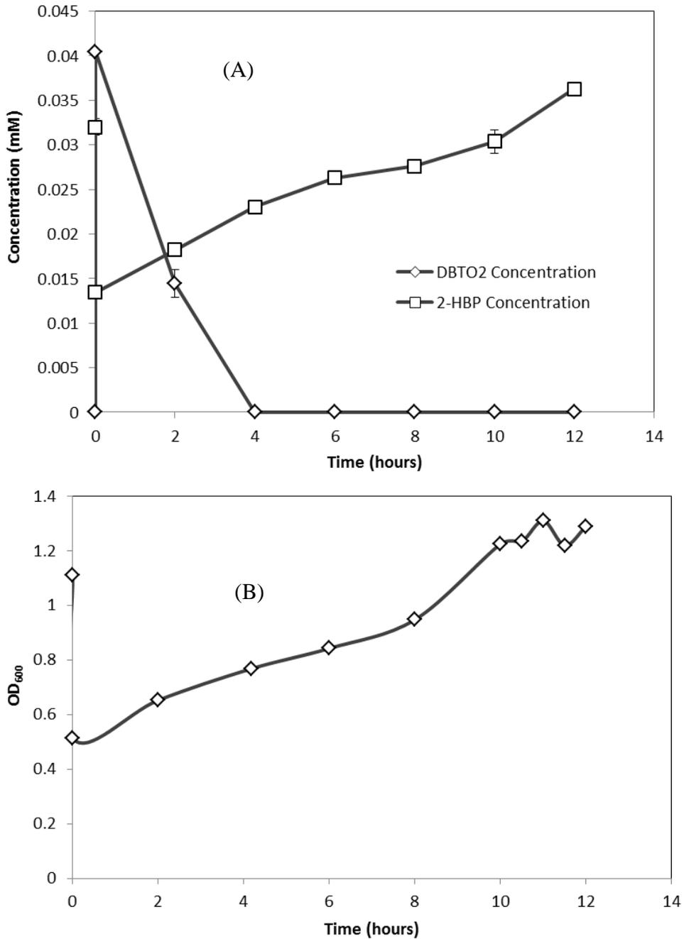
**Figure 4-25** 2-HBP accumulation (□) and DBTO<sub>2</sub> depletion (◇) (A) and optical density values (B) for cycle 36 of *R. rhodochrous* IGTS8 grown in the SCF with 0.25mM DBTO<sub>2</sub> and 14mM DMFA
