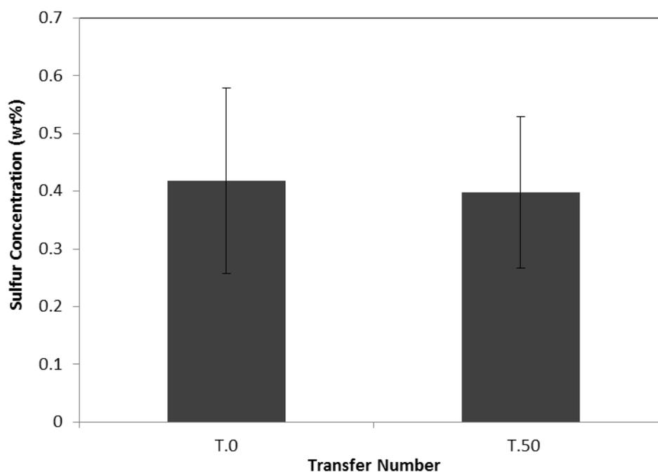
**Figure 4-19** Sulfur elemental analysis results for the original inoculum of *R. rhodochrous* IGTS8 and transfer number 50 in SFMM with 0.25mM DBTO<sub>2</sub> and 14mM DMFA
