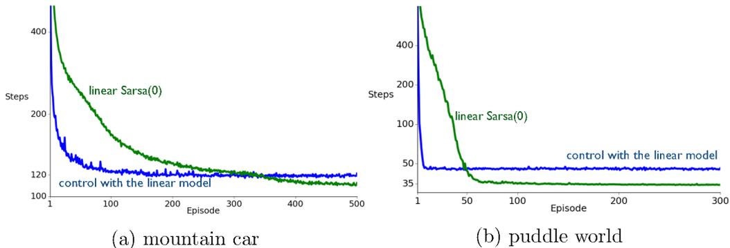
Figure 3.2: Comparison between linear Sarsa(0) and control with the linear model when same computational resources are given to both of the algorithms. In both domains, the model-based algorithm outperforms the model-free algorithm on the early episodes, but reaches to a poor asymptotic performance. The results are for the optimal parameters and are averaged over 500 runs.
