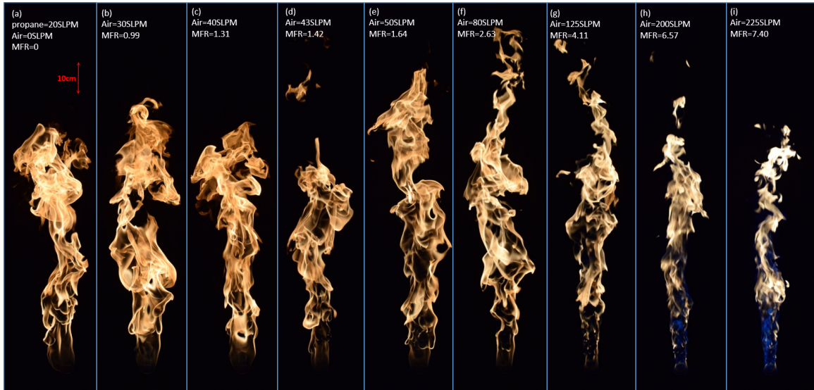
Figure C.3: Instantaneous images of the flame for the 20prCO 2 -TwoOne-fuel100percent case (base case) (also provided in section 3.1)
