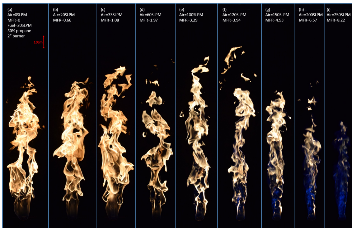
Figure C.9: Instantaneous images of the flame for the 20prCO 2 -TwoOne-fuel50percent case
