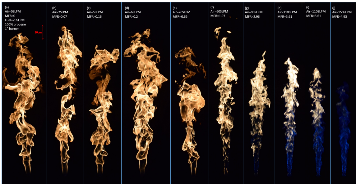
Figure C.5: Instantaneous images of the flame for the 20prCO 2 -OneHalf-fuel100percent case
