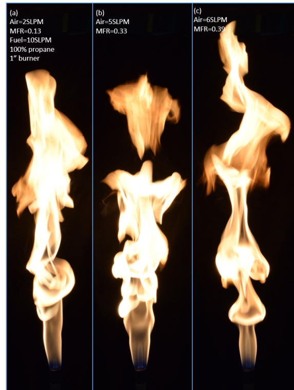
Figure C.2: Long exposure images of 10 SLPM pure propane flame on 1" burner. The inner flame is lifted just before blow-off (c)
