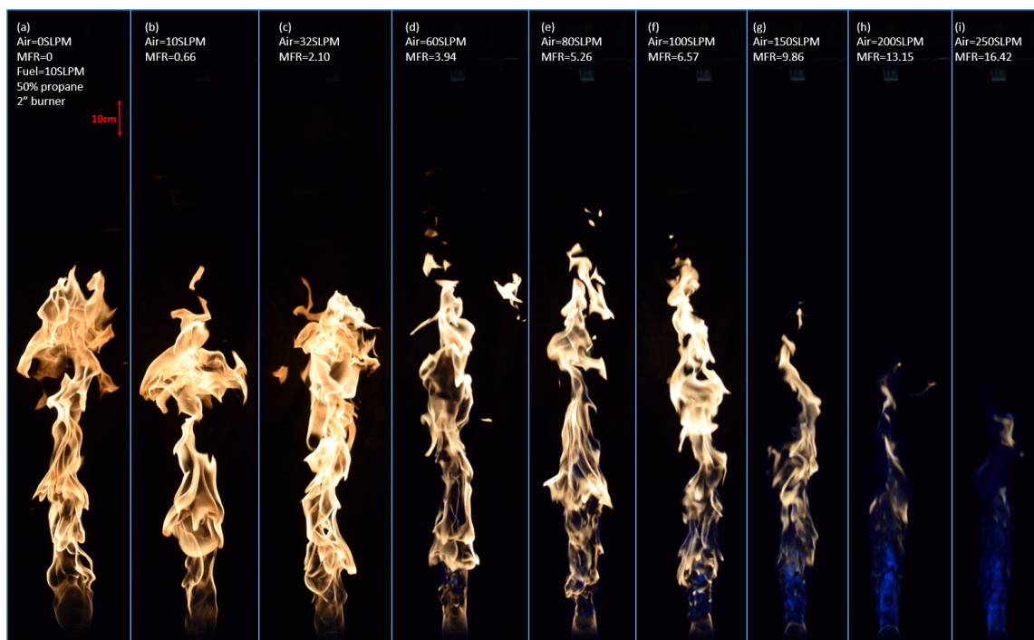
Figure C.10: Instantaneous images of the flame for the 10prCO 2 -TwoOne-fuel50percent case
