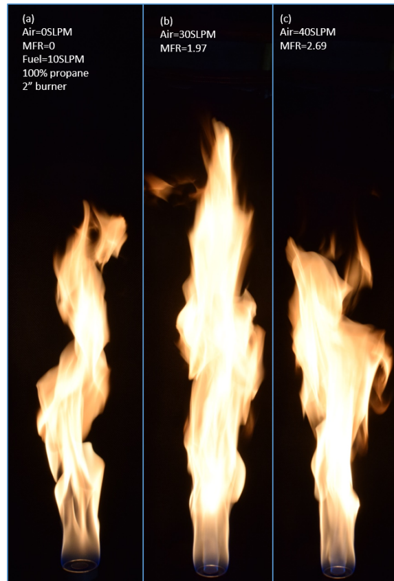
Figure 3.1: Long exposure flame images for 10 SLPM pure propane on 2” burner case before inner flame blow-off. Refer to Appendix C for more select long exposure pictures of flames with an inner flame
