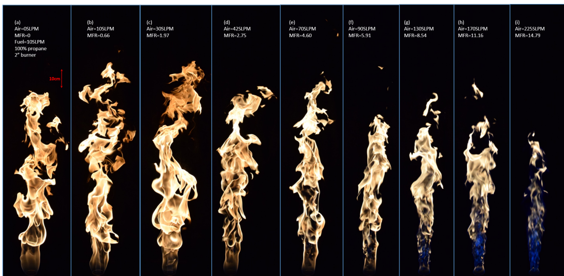
Figure C.4: Instantaneous images of the flame for the 10prCO 2 -TwoOne-fuel100percent case
