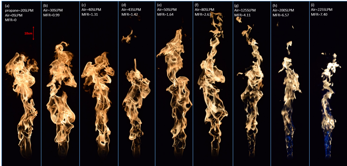
Figure 3.2: Instantaneous images of the flame for the base case. A pale radiance of the inner flame attached to the inner tube is visible for MFR=0.99 and 1.31 . Assist flow is increased from left to right. The inner flame is blown off at MFR=1.42 . For instantaneous images of all other cases refer to Appendix C.
