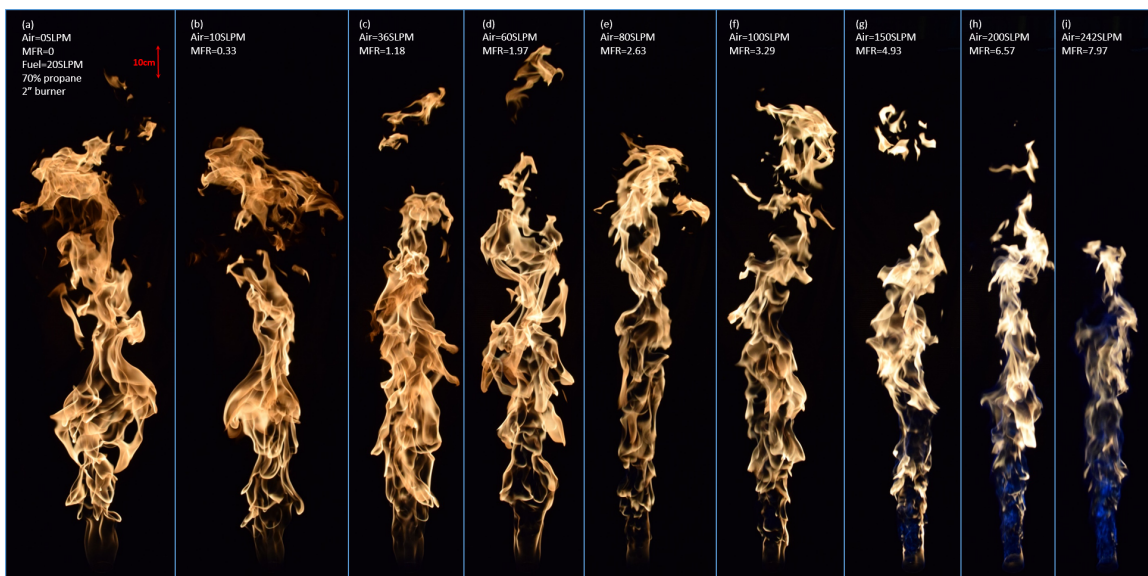
Figure C.7: Instantaneous images of the flame for the 20prCO_2 -TwoOne-fuel70percent case
