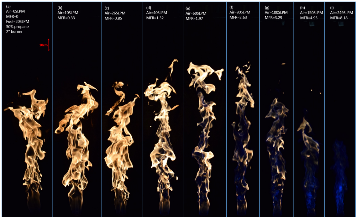
Figure C.11: Instantaneous images of the flame for the 20prCO2-TwoOne-fuel30percent case
