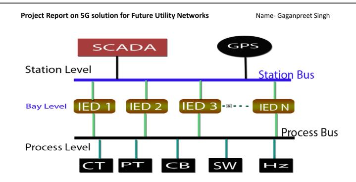
Fig 16 – 61850 Three level architecture
