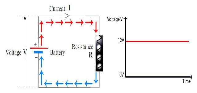
Fig 3 – A simple DC electrical Circuit
