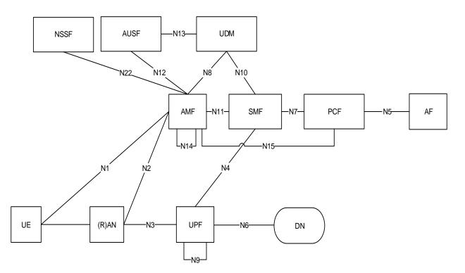
Fig 42–[32] 3GPP 5G system architecture (non-roaming)
