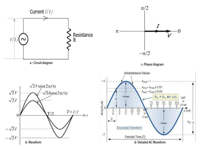
Fig 4 – [1] A simple AC electrical circuit and waveform
