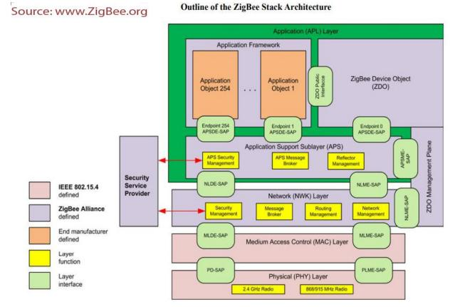
Fig 21 – [17] Zigbee architecture
