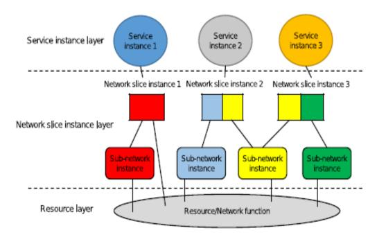
Fig 36- [29] Component of network slicing
