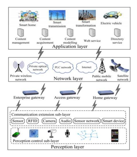
Figure 51 – [39] Three layered architecture for IoT-aided 5G systems
