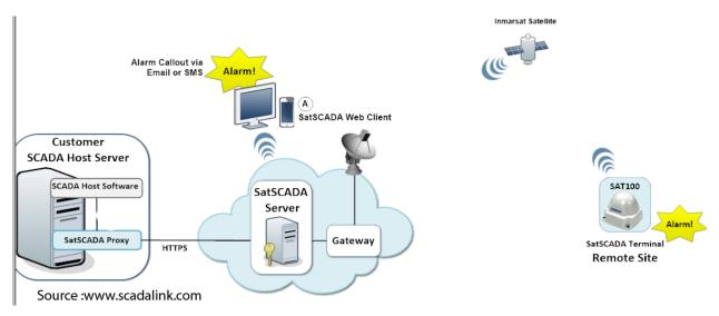
Fig 22 [18] SCADA communication via Satellite
