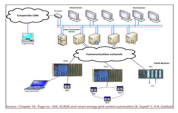
Fig 14 – [8] SCADA IED, RTU, PLC
