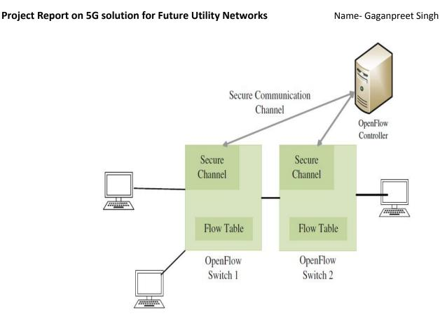
Figure 32 – [26] Open Flow architecture
