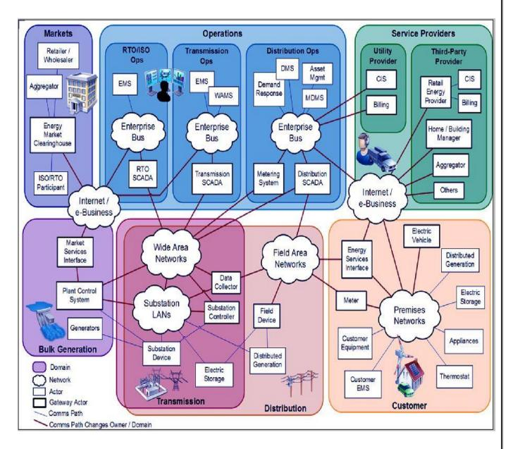
Fig 11 – [5] Smart Grid Information Network - (Logical Model of Legacy Systems Mapped onto Conceptual Domains)
