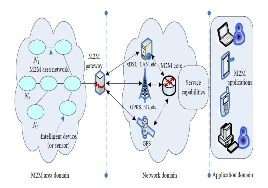
Figure 46: [35] Architecture of M2M networks
