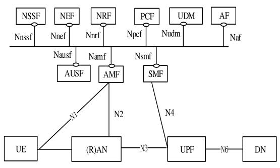
Fig 41– [32] Service based interfaces 5G system architecture (non-roaming)
