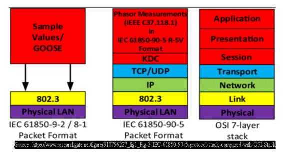
Fig 19 - [13] IEC 61850-90-5 protocol stack compared with OSI stack
