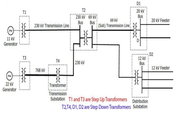
Fig 6 [3] Transmission system line diagram
