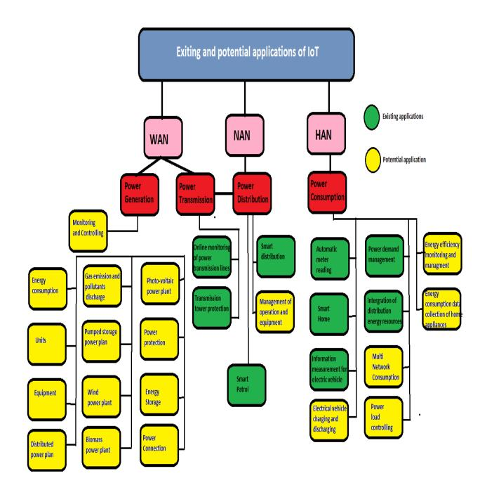
Figure 50- [39] Applications of IoT aided Smart Grid systems
