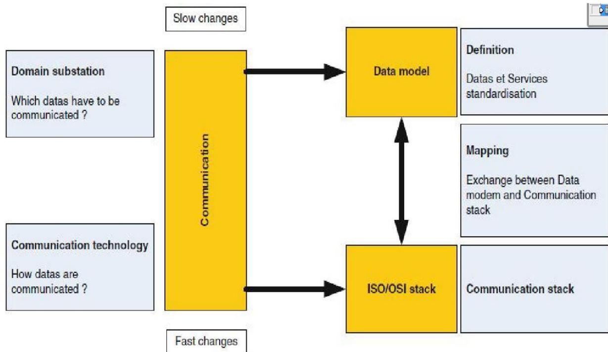
IEC 61850 model presenting data model and communication stack
