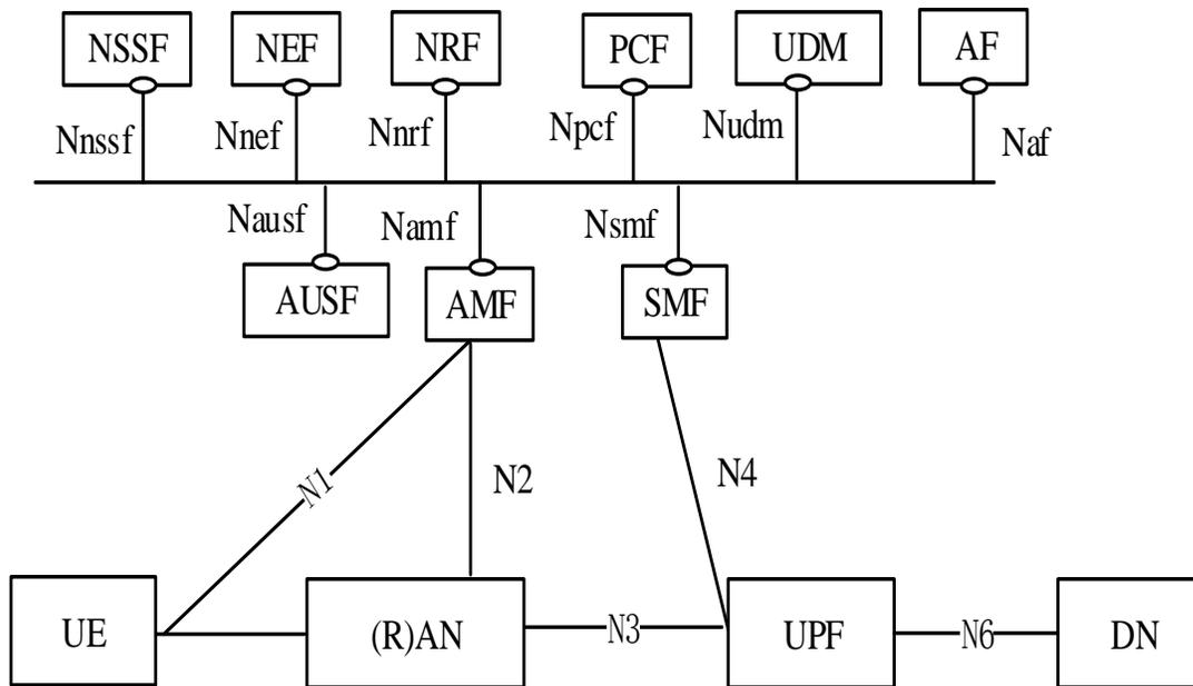
Fig 41– [32] Service based interfaces 5G system architecture (non-roaming)
