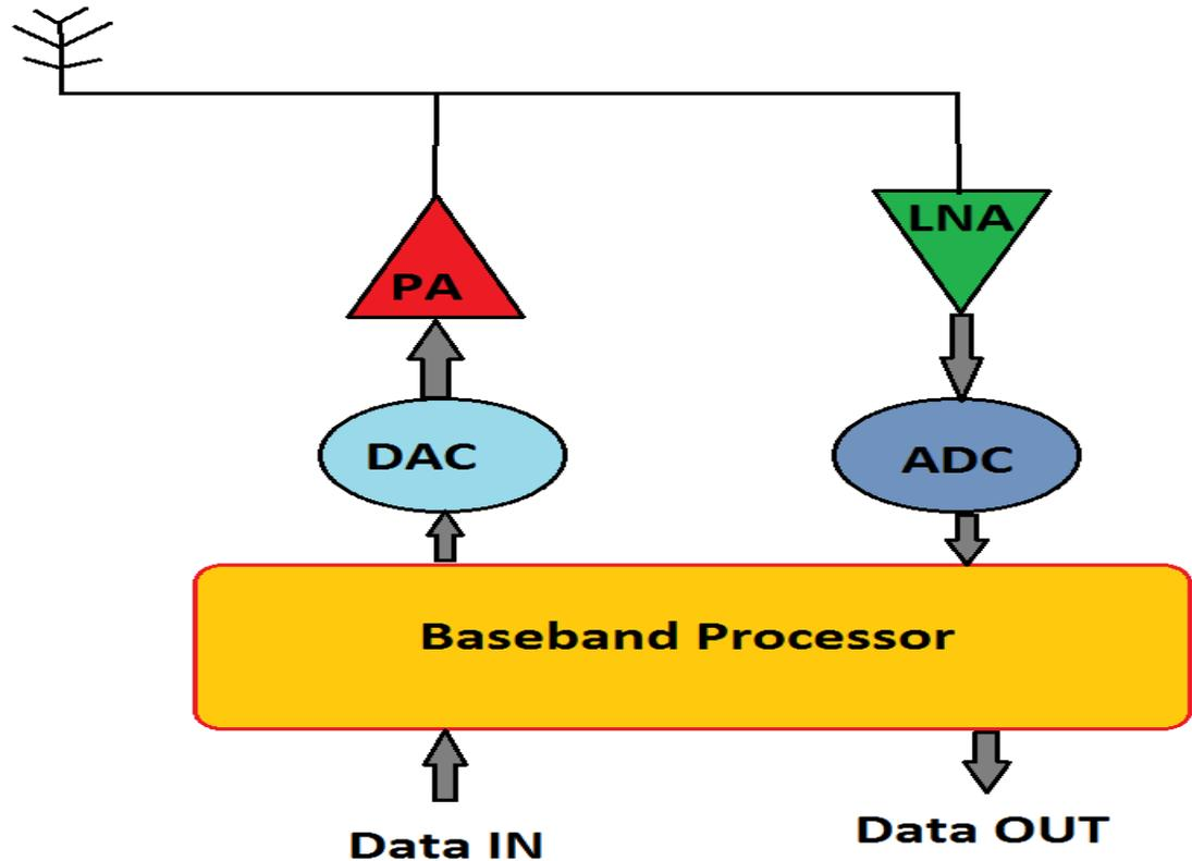
**Fig 34 – Block diagram of an 'Ideal' Software Defined Radio**
