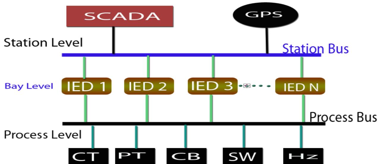
Fig 16 – 61850 Three level architecture
