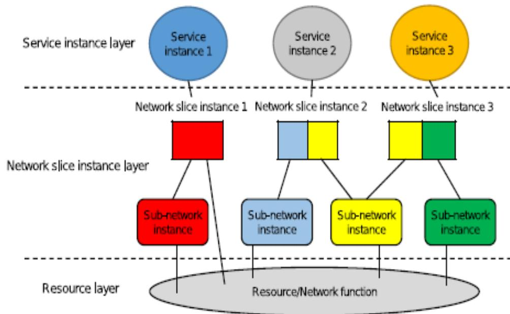
Fig 36- [29] Component of network slicing
