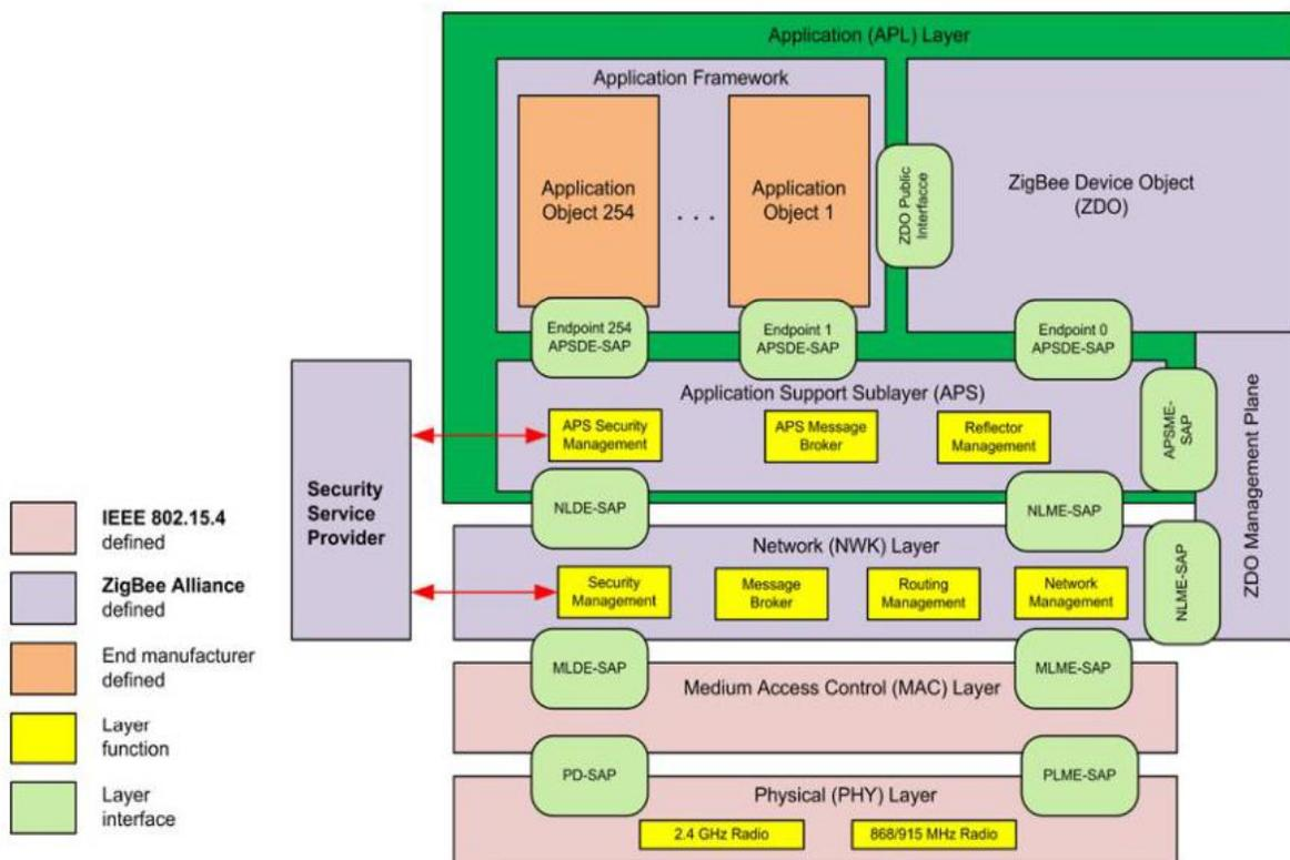
Fig 21 – [17] Zigbee architecture
