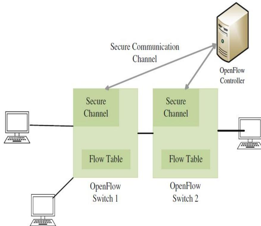
Figure 32 – [26] Open Flow architecture
