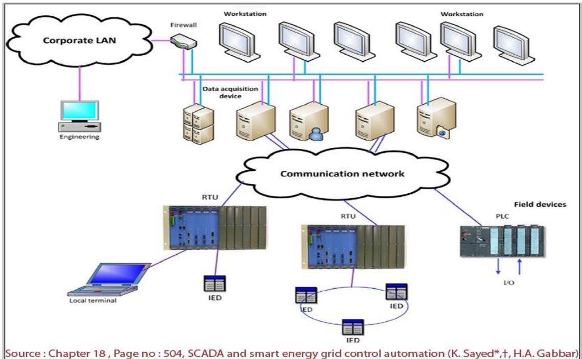
Fig 14 – [8] SCADA IED, RTU, PLC
