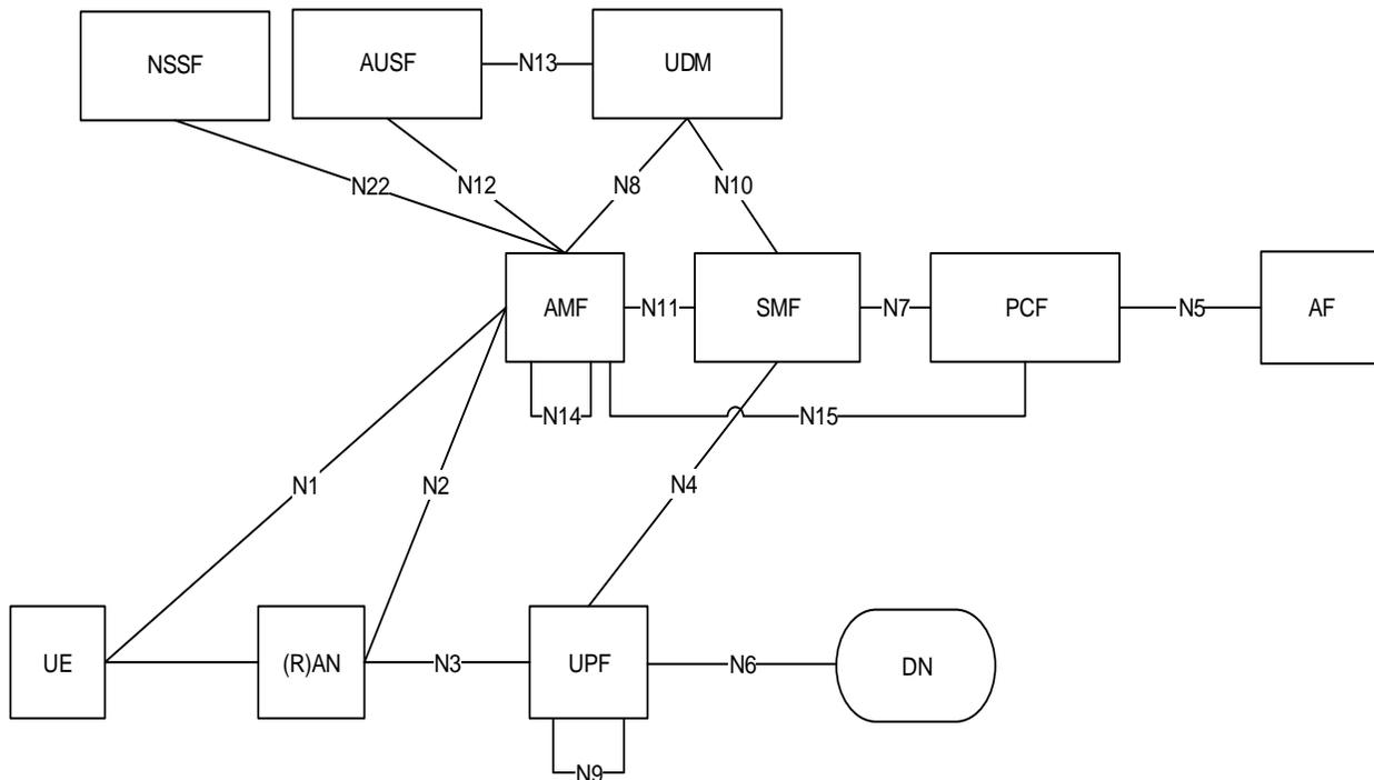
Fig 42– [32] 3GPP 5G system architecture (non-roaming)
