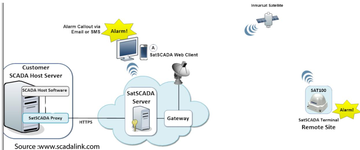
Fig 22 [18] SCADA communication via Satellite
