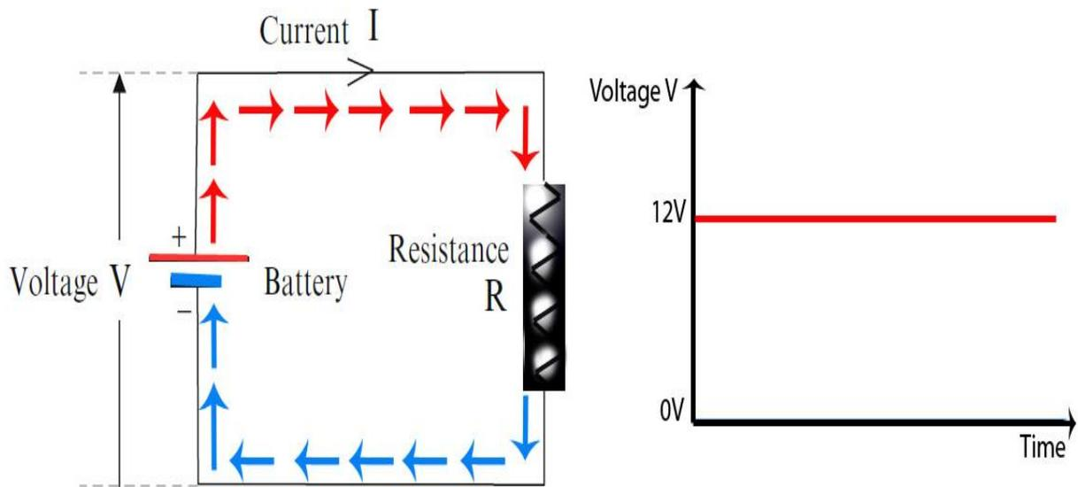
Fig 3 – A simple DC electrical Circuit
