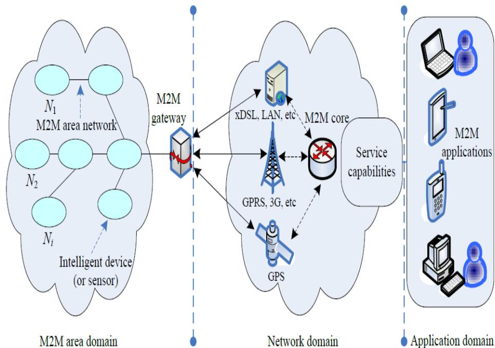
Figure 46: [35] Architecture of M2M networks
