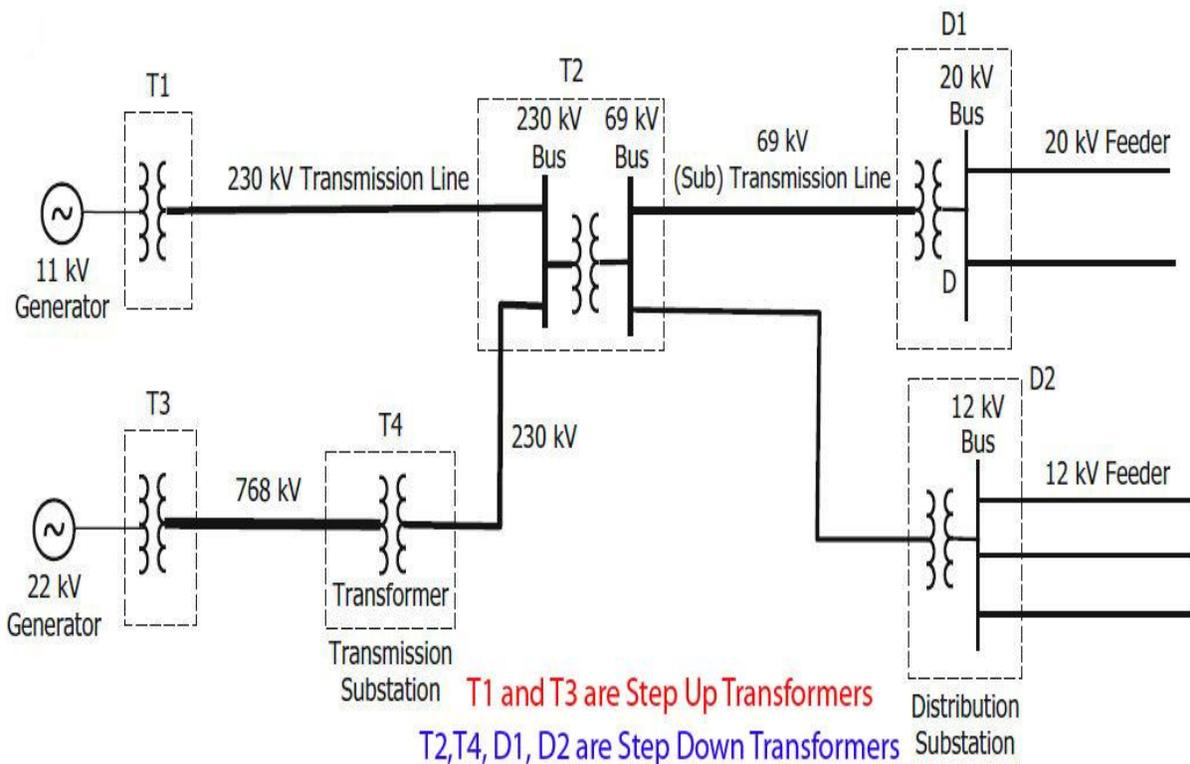
Fig 6 [3] Transmission system line diagram
