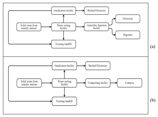
Figure 28: (a) Flow of waste from transfer stations to an integrated gasification and anaerobic digestion facility, (b) Flow of waste from transfer stations to an integrated gasification and composting facility
