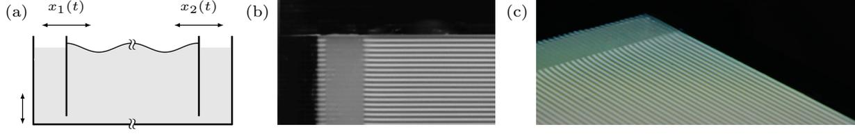
**Figure 2.2:** (a) A cross-section of a rectangular container with two moving walls on the left and right; the entire container moves vertically in time. Top (b) and side (c) views of static contact angle near a corner of the domain; the length scale is set by the thickness of the wall being 12.7 mm.
