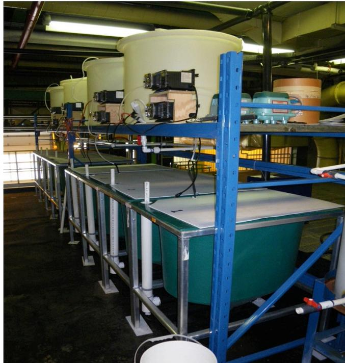
**Figure 3.1:** The real time exposure apparatus system located at the Oil Sands Research Innovation facility in Devon, AB. OSPW is pumped to the 300 L header tanks (white). From there the water is either pumped straight into the green 150L tanks containing goldfish, or diluted with peristaltic pumps (black). Water is renewed at a flow rate of 75L/ day.
