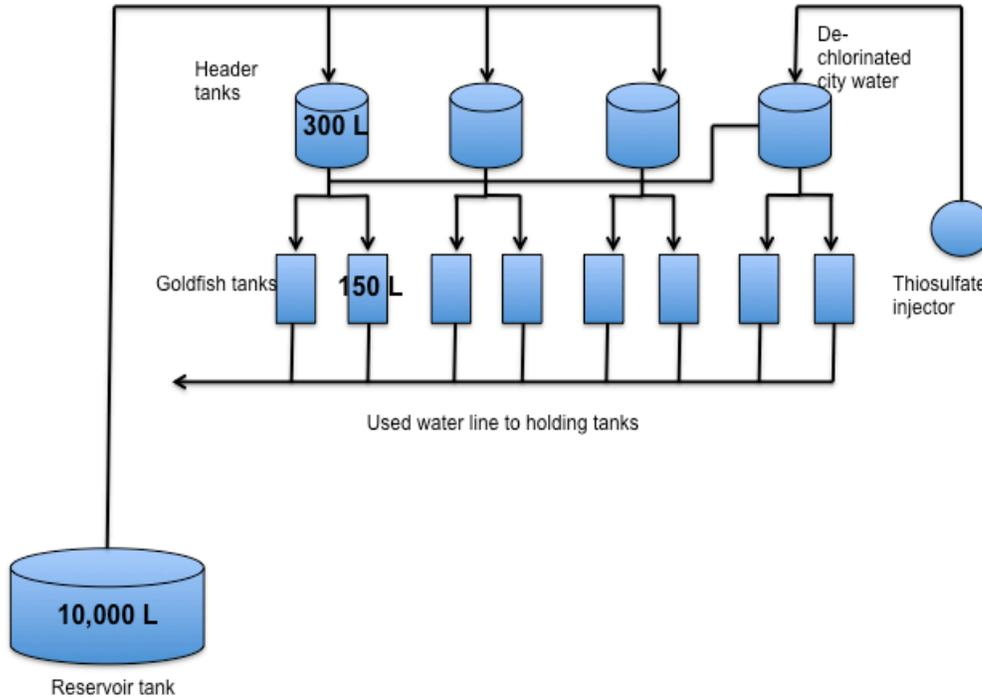
**Figure 3.2:** A schematic drawing of the real time flow through experimental setup at the Oil Sands Research Innovation facility in Devon, AB. OSPW was pumped from the 10,000L reservoir tank to 300L header tanks. The water was then either pumped directly, or diluted with thiosulfate injected city water, to 150L goldfish holding tanks. Each tank had a flow-through rate of 75L/ day and the used OSPW was stored in two 5000 L holding tanks (not shown).
