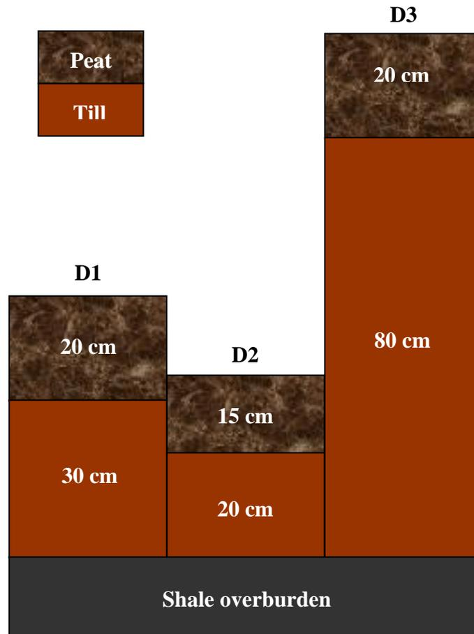
Figure 17. Depth of peat and till in the D1, D2 and D3 prototype covers on SW30 Dump (Shurniak 2003 and Rodger 2008).
