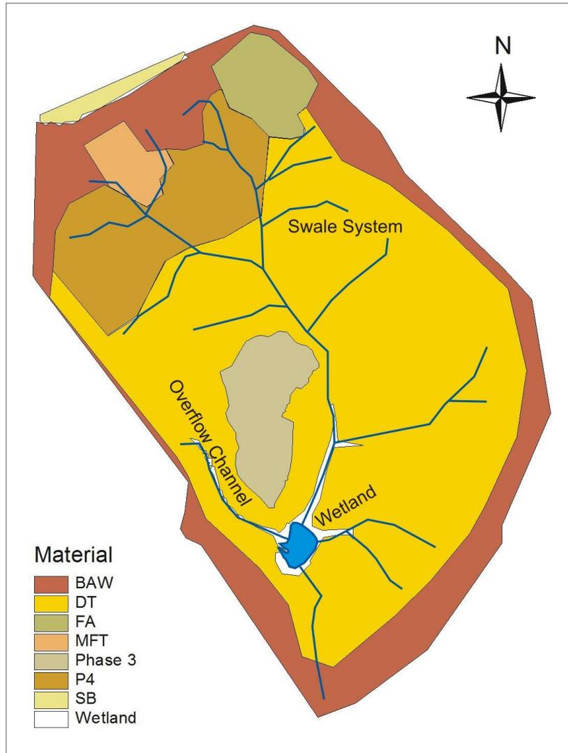
Figure 91. Distribution of materials used in the construction of Wapisiw Lookout watershed (Suncor n.d.).
