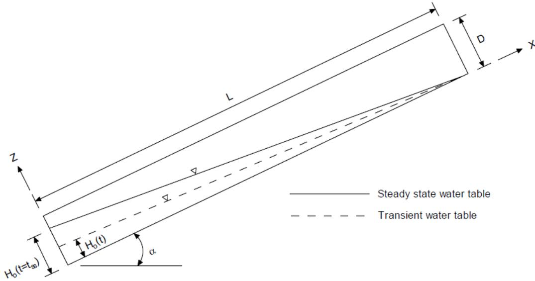
Figure 4. The kinematic storage model (Sloan and Moore 1984).
