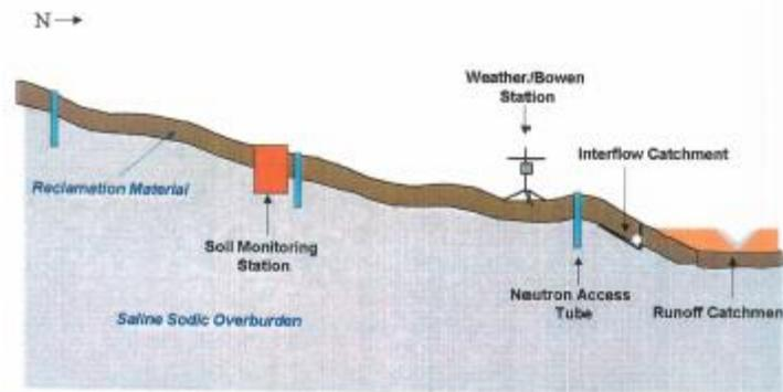
Figure 20. Cross section of the SW30 Dump prototype covers showing the position of the instruments in the landscape (Boese 2003).
