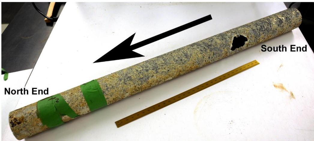
Figure A-23: As collected north section of removed tubular tie. Arrow points north and scale is 300 mm.
