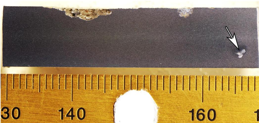
Figure A-74: Overall image of the etched floor cross-section. The mark near the bottom right corner (white arrow) is an artifact from the etching process. Scale is in mm.
