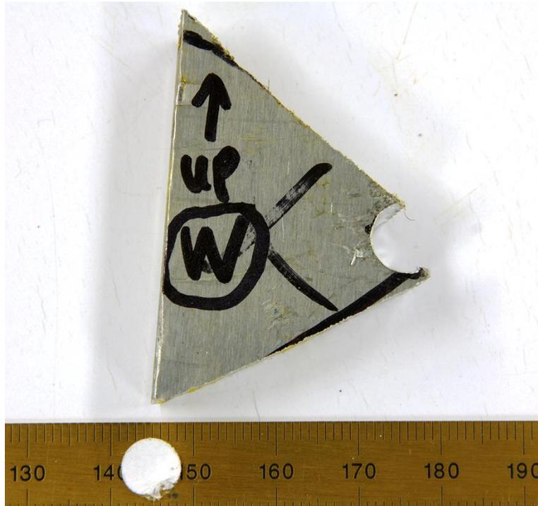
Figure A-14: Wall section collected from aeration tank. Scale is in mm.
