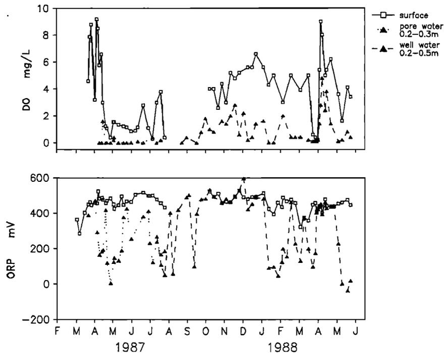
Fig. 3. Temporal variation in (top) dissolved oxygen concentration (DO) and (bottom) oxidative reduction potential (ORP) of surface and peat pore or well water at swamp site 1 for March 1, 1987 to May 31, 1988.
