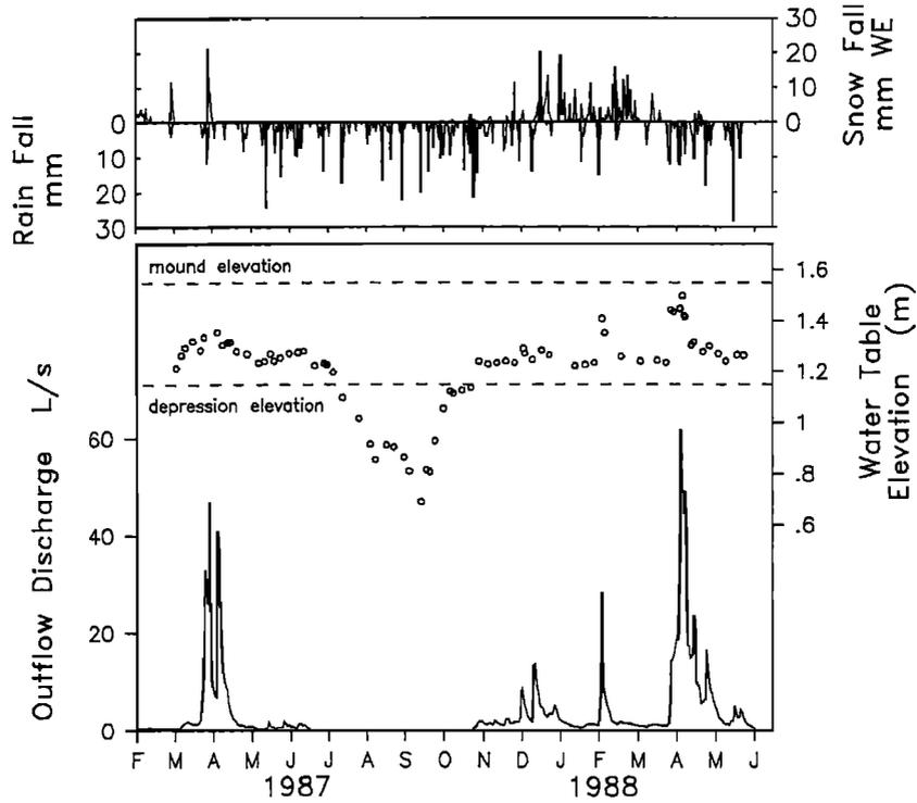
Fig. 2. Daily rain and snowfall depths, swamp outflow discharge, and water level elevation at swamp site 1, for March 1, 1987, to May 31, 1988.
