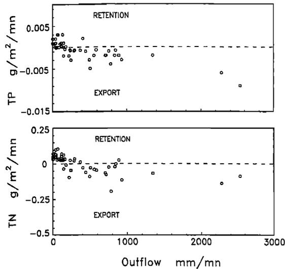
Fig. 6. Monthly total phosphorus (TP) and total nitrogen (TN) retention versus outflow runoff of Plastic I swamp from June 1984 to May 1988. All budgets calculated by prorating unit runoff (see text).
