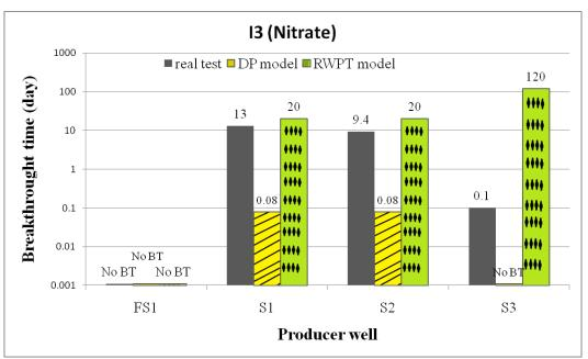
Figure 3-17. Comparison of breakthrough times obtained through field test and two different modeling approaches for injector I3.
