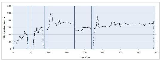
Figure 4-23.  $CO_2$  injection rate (re-produced from Baxter, 1990).  $CO_2$  injection period is divided into 8 smaller sub-periods.
