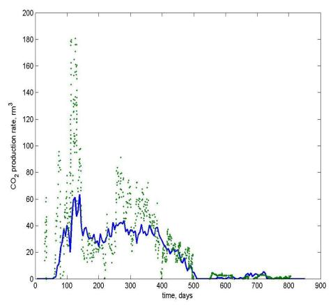
Figure 4-24. Best history match for the model, where  $CO_2$  injection is represented by eight periods of injection at constant rate. Dots: observed data; solid line: simulated data.
