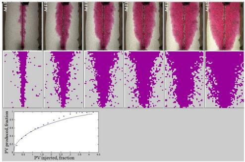
Figure 2-9. Experimental and simulation results for horizontal light oil displacement at 45 ml/hr.
