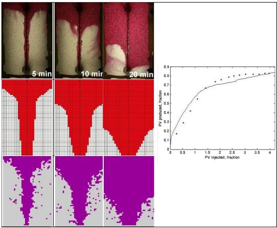
Figure 2-11. Vertical light oil displacement at 45 ml/hr.
