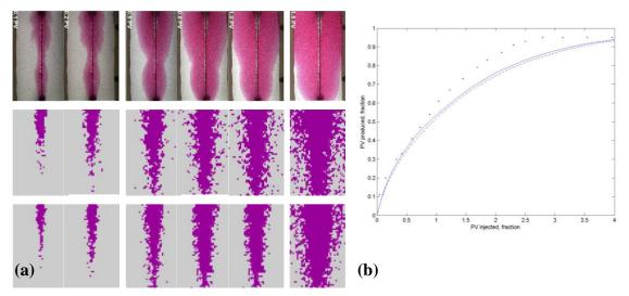
Figure 2-3. Comparison of experimental data given by Er (2009) with results of simulation using 15\*40\*1 grid and 31\*80\*1 grid.
