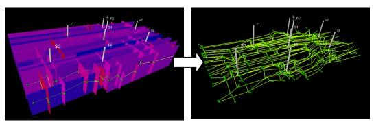
Figure 3-2. Graph created based on fracture network.
