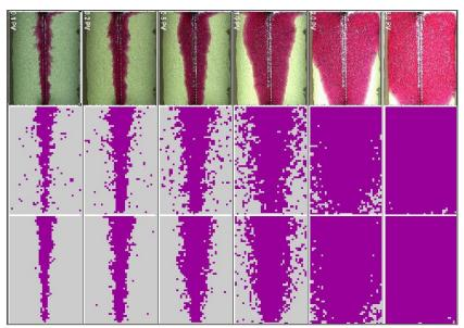
Figure 2-5. Comparison of experimental visual data with results of simulation using 16 and 36 walkers per grid cell.
