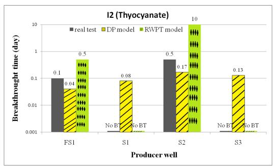
Figure 3-16. Comparison of breakthrough times obtained through field test and two different modeling approaches for injector I2.
