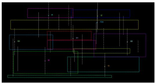
Figure 3-9. Midale  ${\rm CO_2}$  pilot area divided into blocks for modeling. Rectangular blocks are to be populated by on-trend fractures. Off-trend fractures are shown by grey vertical lines.
