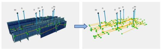
Figure 4-2. Graph created based on fracture network. Vertexes are added at fracture ends and fracture intersections (green spheres). Edges are added between connected vertexes (yellow lines). Only this graph is used for further simulation.
