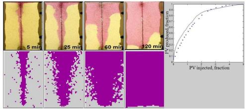
Figure 2-13. Experimental and simulation results for vertical heavy oil displacement at 15 ml/hr.
