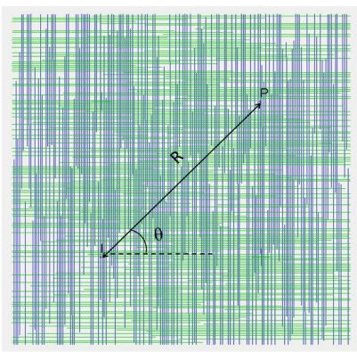
Figure 5-6. Fracture network consisting of two mutually perpendicular fracture sets. Lengths of all fractures are nearly equal.
