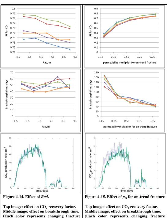
Top image: effect on  $CO_2$  recovery factor. Middle image: effect on breakthrough time. (Each color represents changing fracture spacing for one fracture network realization.) Bottom image: effect on  $CO_2$  production rate. Green solid line  $-p_m$ =0.6; blue dotted line  $-p_m$ =1. Other parameters do not change.
