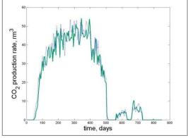
Figure 4-9. Effect of on-trend fracture permeability.
