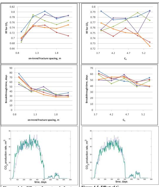
Figure 4-4. Effect of on-trend fracture spacing.
