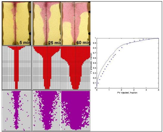
Figure 2-12. Vertical heavy oil displacement at 15 ml/hr.
