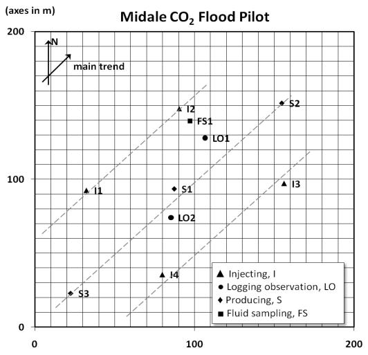
Figure 3-4. Midale CO<sub>2</sub> Flood Pilot configuration (After Bogatkov, 2008).
