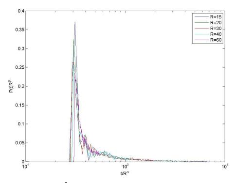
Figure 5-12. Plotting  $P(t)R^{\beta}$  vs.  $t/R^{\alpha}$  overlays all curves reasonably well even when we use approximate values for scaling parameters. Values of scaling parameters obtained using trends from Figures 8a and 8b are:  $\alpha$ =1.79;  $\beta$ =1.55.
