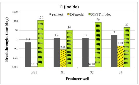
Figure 3-15. Comparison of breakthrough times obtained through field test and two different modeling approaches for injector I1.
