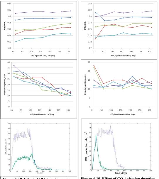
Figure 4-18. Effect of CO<sub>2</sub> injection rate.
