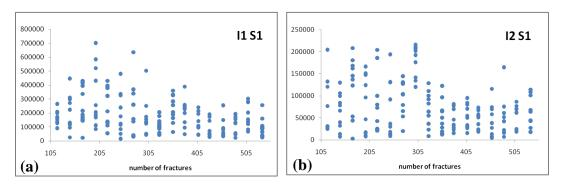
Figure 3-5. Simulation result vs. number of fractures. The value in the y-axis indicates the difference between cumulative tracer production curves for different stochastic realizations. Figure (a) shows result for injector I1 and producer S1; Figure (b) shows result for injector I2 and producer S1.
