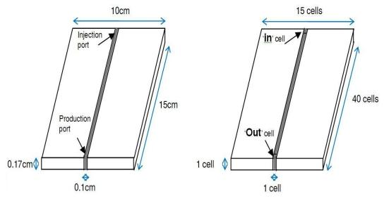
Figure 2-2. Sketches of the experimental (left) and simulation (right) models.
