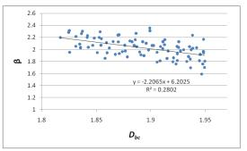
Figure 5-10.  $\alpha$  and  $\beta$  vs. fracture network box-counting fractal dimension.
