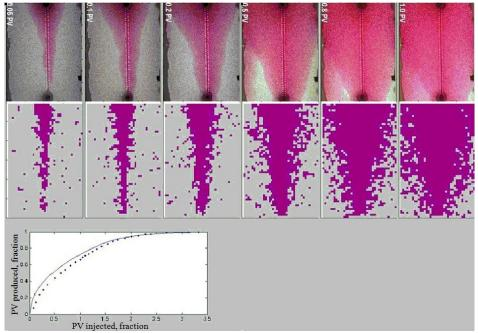
Figure 2-7. Experimental and simulation results for horizontal kerosene displacement at  $15 \, \text{ml/hr}$ .
