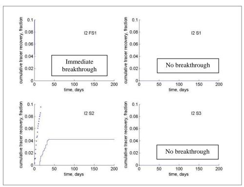
Figure 3-11. History match of tracer tests for injector I2. Dots: observed tracer recovery; line: simulated tracer recovery.
