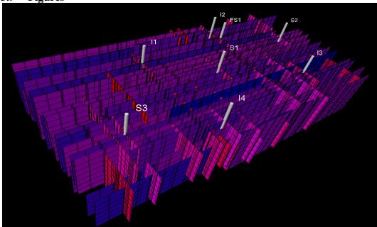
Figure 3-1. Fracture network represented by classical simulation grid.
