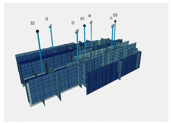
Figure 4-1. Fracture network represented by a classical simulation grid. Only high permeable (fracture) cells are shown. Color shows permeability of each fracture.
