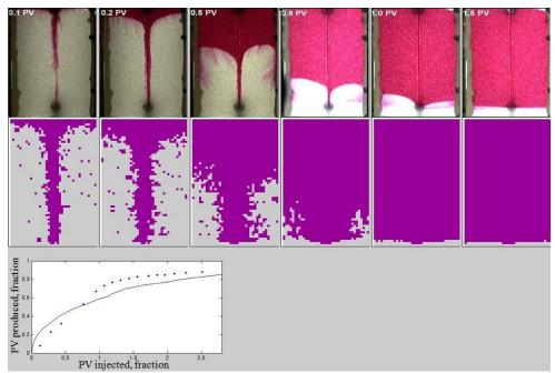
Figure 2-10. Experimental and simulation results for vertical light oil displacement at 15 ml/hr.
