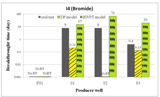
Figure 3-18. Comparison of breakthrough times obtained through field test and two different modeling approaches for injector I4.
