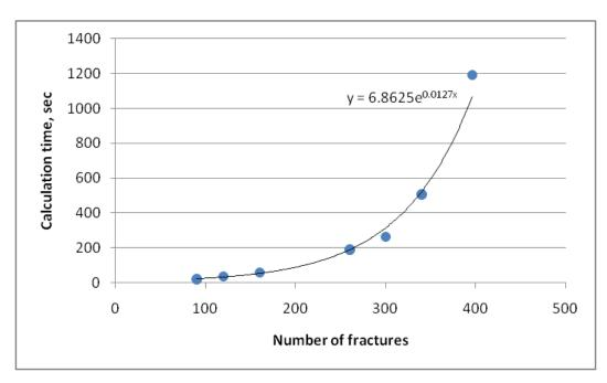
Figure 3-19. Calculation time for different fracture networks.
