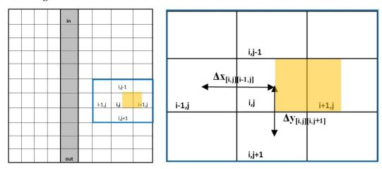
Figure 2-1 Schematic of the Random Walk simulation model. Oil and solvent walkers in shaded (yellow) area are counted to calculate viscosity between cells [i,j] and [i+1,j].
