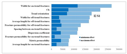
Figure 3-8. Effect of parameters for injector I2 and producer S1.
