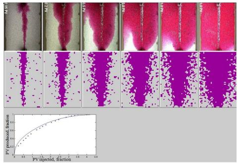
Figure 2-8. Experimental and simulation results for horizontal light oil displacement at 25 ml/hr.
