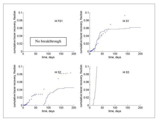
Figure 3-13. History match of tracer tests for injector I4. Dots: observed tracer recovery; line: simulated tracer recovery.
