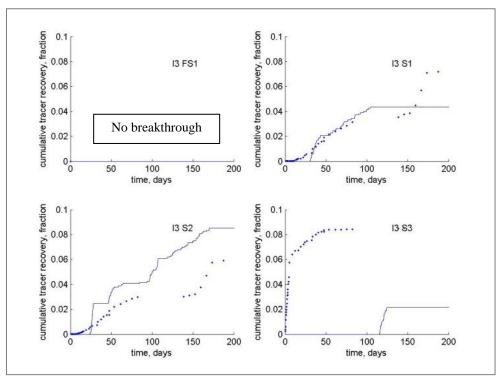
Figure 3-12. History match of tracer tests for injector I3. Dots: observed tracer recovery; line: simulated tracer recovery.
