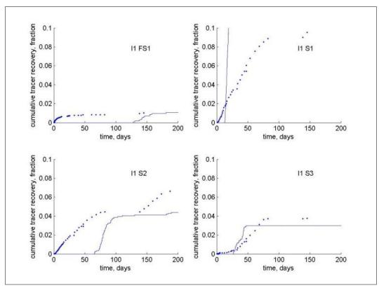
Figure 3-10. History match of tracer tests for injector I1. Dots: observed tracer recovery; line: simulated tracer recovery.
