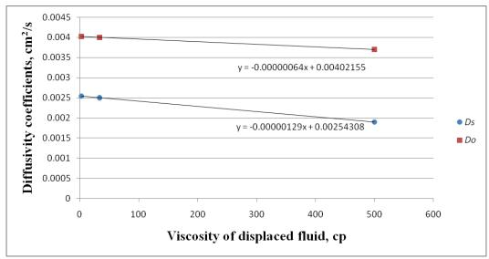
Figure 2-14. Correlation between oil and solvent diffusivity coefficients and viscosity of displaced fluid for horizontal flow.
