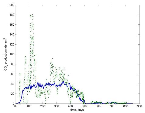
Figure 4-22. Best history match for the model, where  ${\rm CO_2}$  injection is represented by one period of injection at constant rate.
