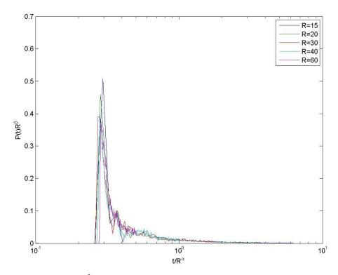
Figure 5-5. Plotting  $P(t)R^{\beta}$  vs.  $t/R^{\alpha}$  overlays all curves.  $\alpha$ =1.8138;  $\beta$ =1.658 for the fracture network used in this particular example.
