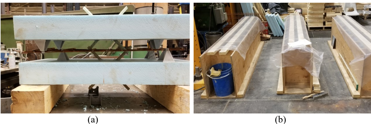
Figure 3.3 (a) Push through assembly showing shear connector and reinforcement arrangement (b) push-through formwork
