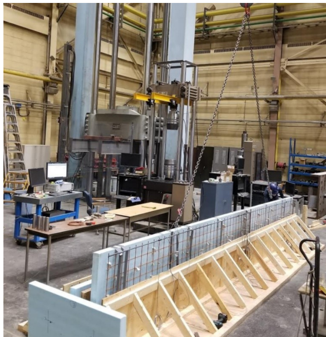
Figure A.4 Formwork preparation of IWP
