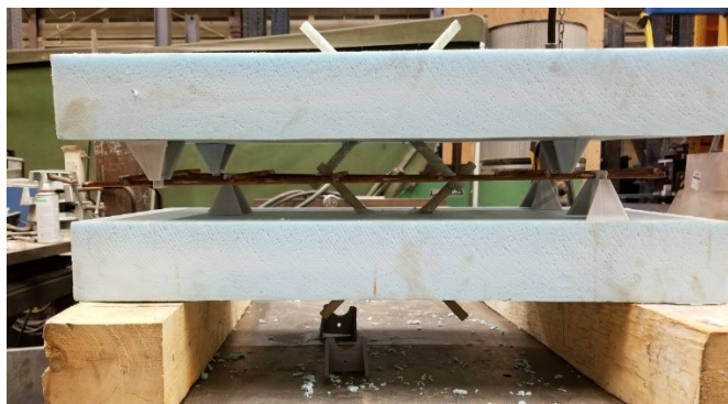
Figure A.2 Push-through specimen preparation
