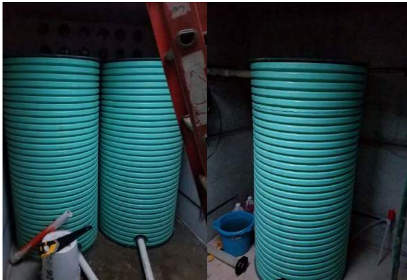
Figure 10. Cylindrical collection basins inside vault for monitoring flows.
