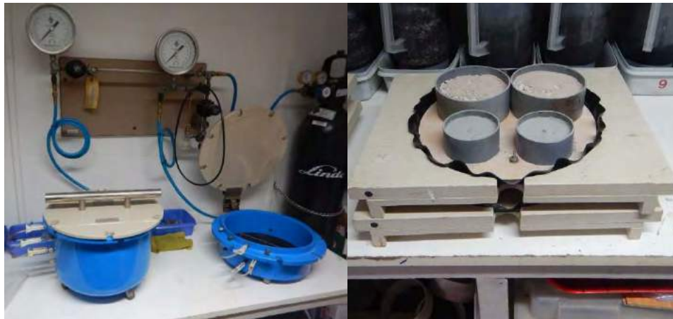
Figure 4. Pressure plate equipment used to obtain SWCC
