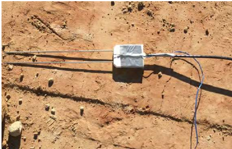
Figure 12. Water content reflectometer with thermocouple taped to head and ready to be deployed.
