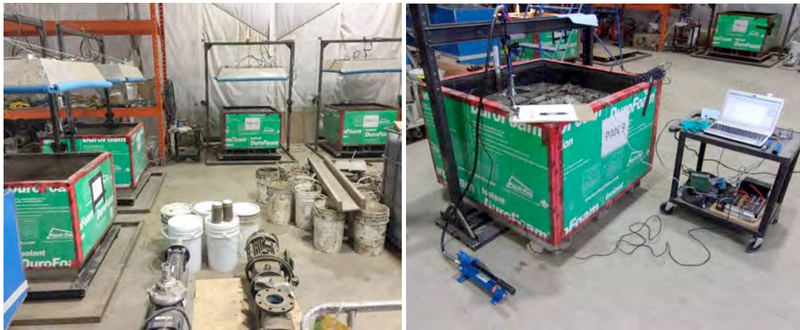
Figure 1. (a) Overview of pans and lab setup. (b) Overall plate load test setup showing pan, reaction frame, hydraulic ram, load cell, LVDT, data acquisition equipment and laptop.
