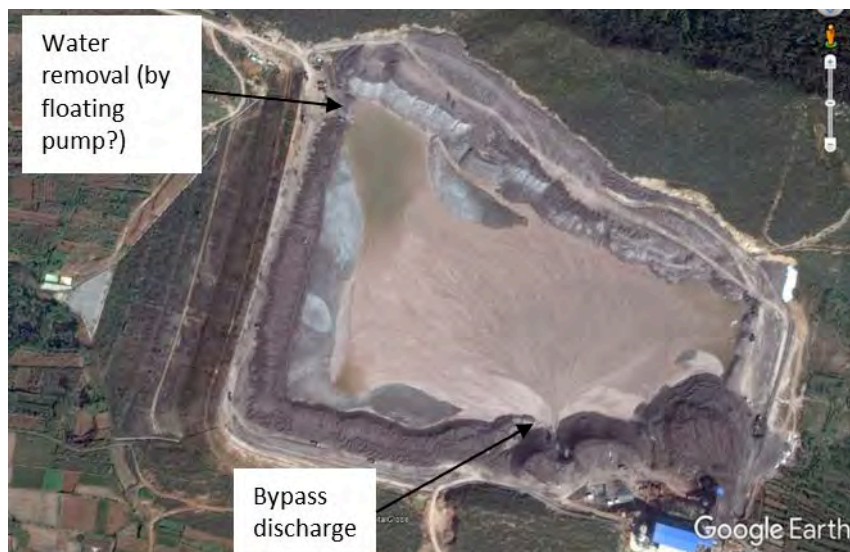
Figure 4. October 2014 – Significant bypass deposition and standing water in north west corner
