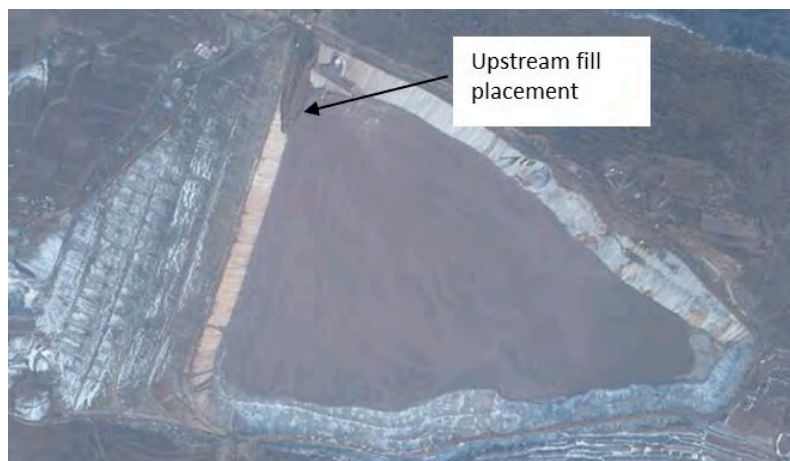
Figure 2. January 2012 – Upstream raising at north end of embankment with thick lift of fill
