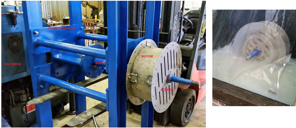
Figure 3. Rotating Drum Ablation Machine for testing logs of clay at the slurry lab of Splitvane Engineers Inc.
