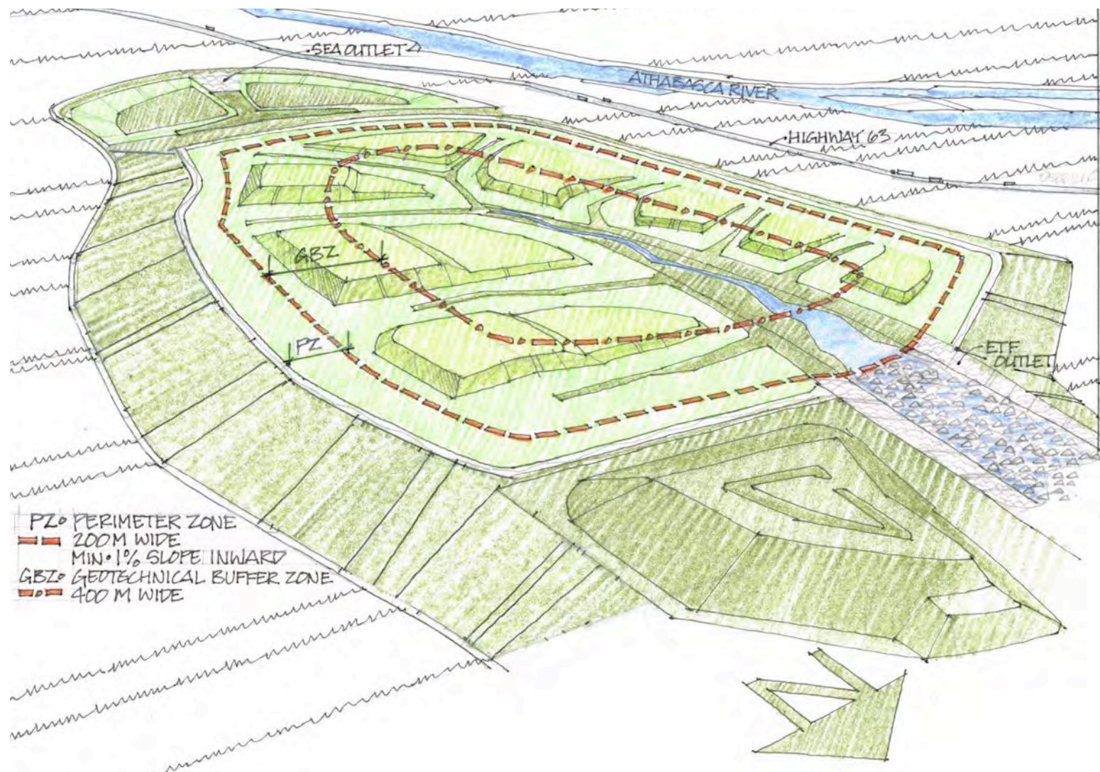
Figure 2: Illustration of the closure landform design for the ETF and SEA. (Illustration by Derrill Shuttleworth)
