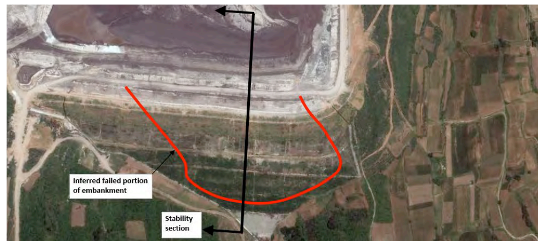
Figure 8. June 2016 geometry, with inferred failure extent and stability section location
