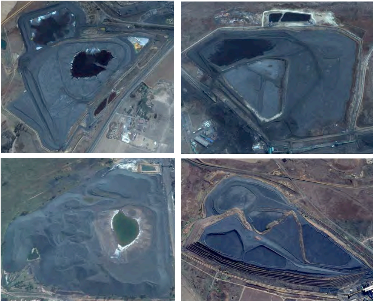
Figure 4. Examples of Fine Tailings Disposal Cells inside Coarse Tailings
