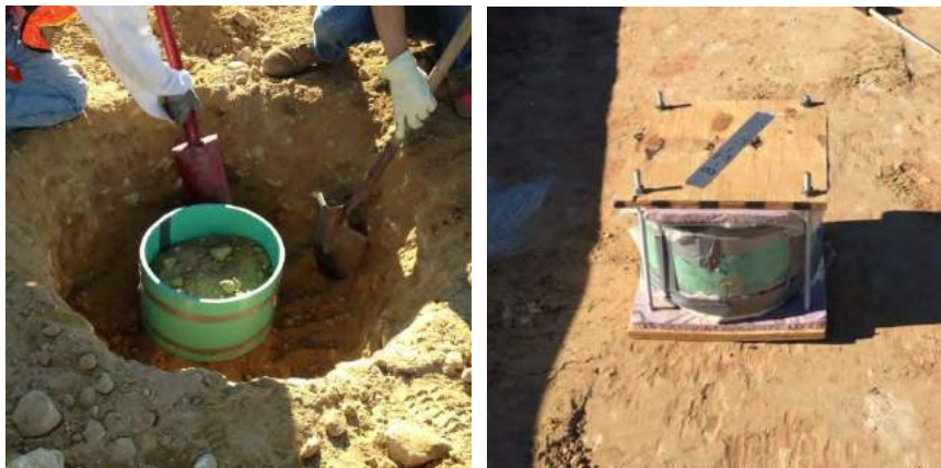
Figure 8. Collecting hand-carved block sample from interim cover layer (left) and block sample in wooden shipping frame for transport to the laboratory (right).
