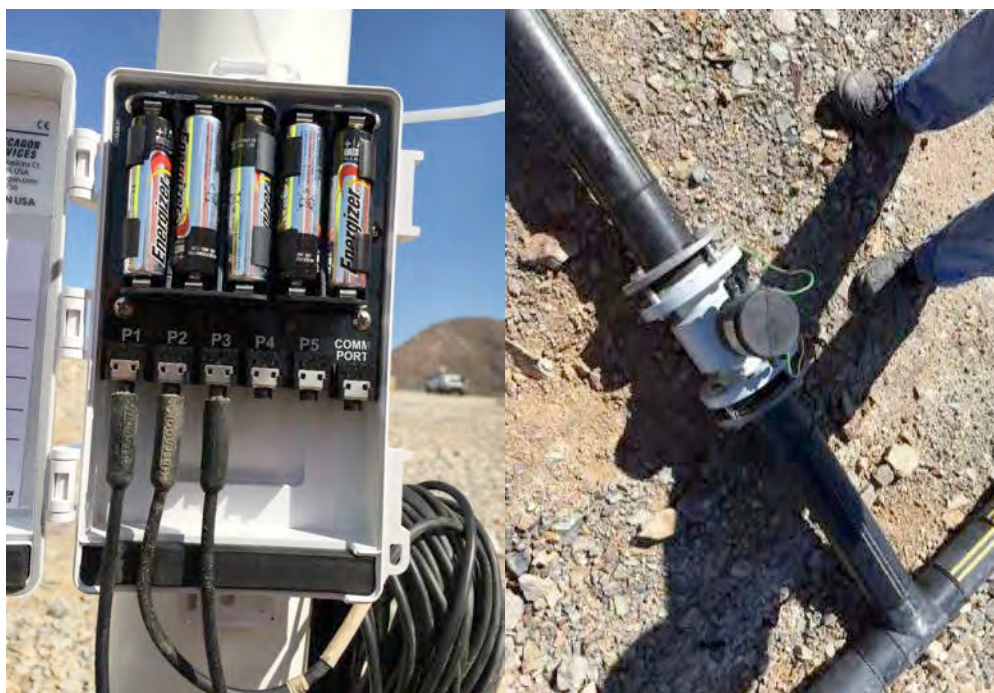
Figure 7 – commercially available moisture sensors and flowmeters to evaluate fluids dispersion through RDA
