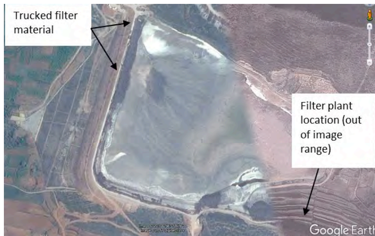
Figure 3. April 2014 – Wall raise construction with using filtered material
