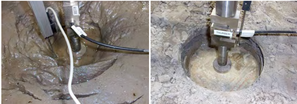
Figure 6. Punching failure observed on the NST in (a) Pan #11 and (b) Pan #08
