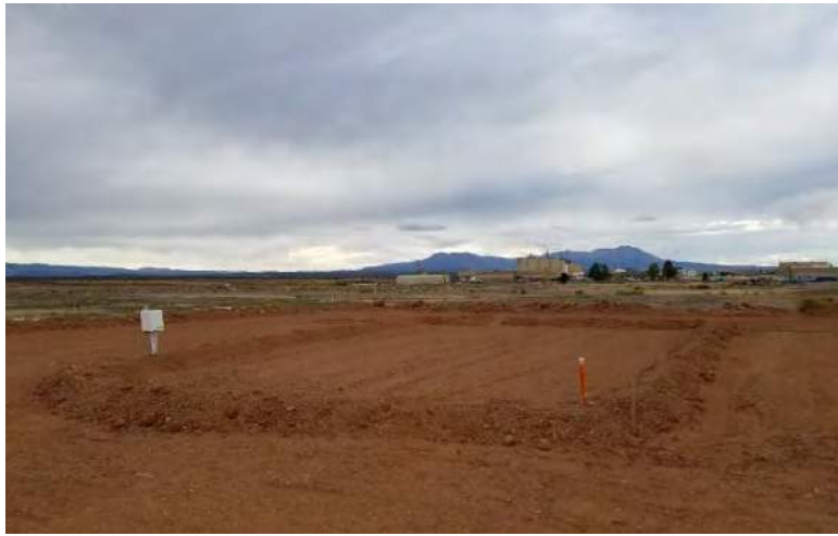
Figure 9. Final surface of test section (looking north) with diversion and collection berms for runoff.
