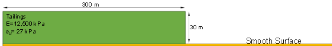
Figure 4. Geometry and material parameters adopted in numerical model.
