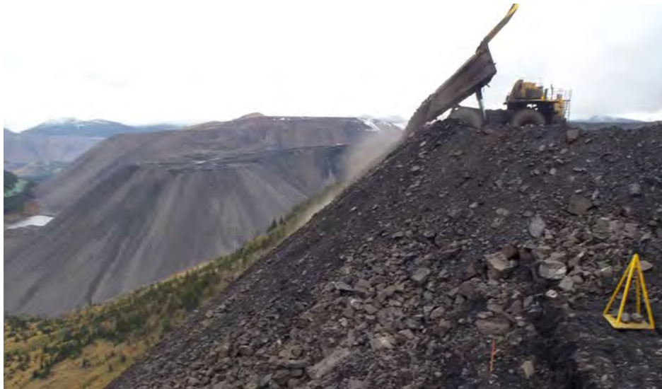
Figure 1. Mine waste dump under active operation, with simple wireline extensometer to monitor ongoing crest displacements.
