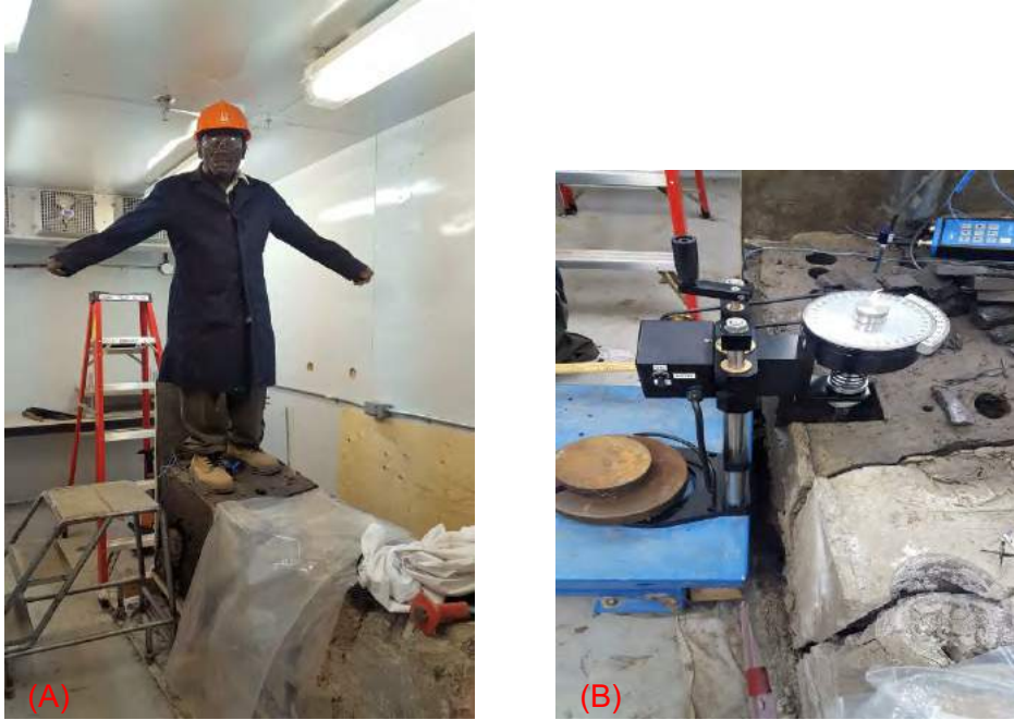
Figure 4. (A) Frozen/Thawed centrifuge product treated under laboratory controlled conditions for 30 months test period and (B) In-situ measurement of shear strength using a vane shear apparatus.
