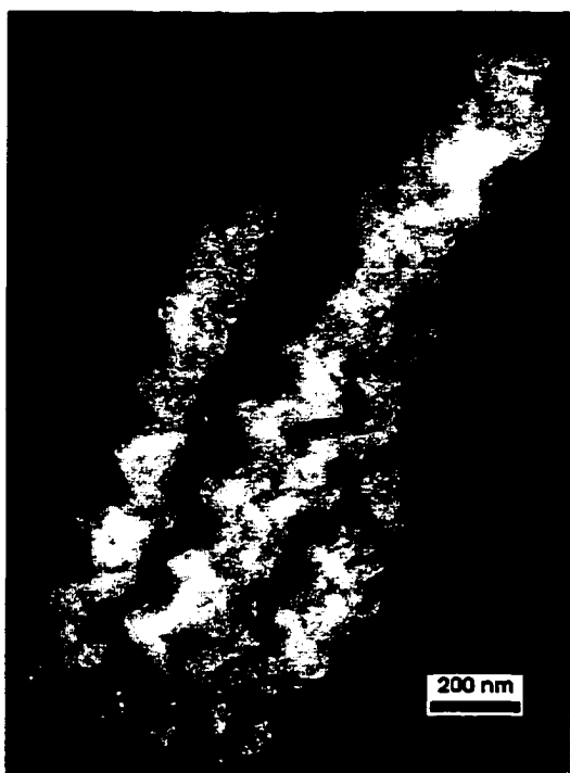
Figure H10 Relation between helices and pillars. Helices are grown by filling helix-pitch. Titanium film grow at \theta = 86^\circ , R = 300 \text{ \AA/s} and \text{RPM} = 1.6 \text{ min}^{-1} . Scale bar corresponds to 200 nm.
