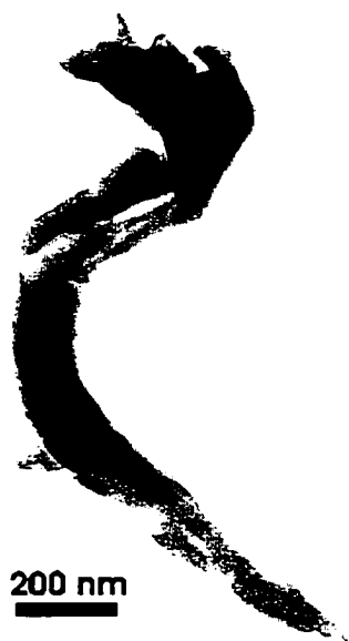
Figure H1 Bifurcation in a bismuth helix. Grown at \theta = 86^\circ , RPM = 0.2 \text{ min}^{-1} , and R = 70 \text{ \AA/s} . Scale bar corresponds to 200 nm. Compare with figure 5.4.
