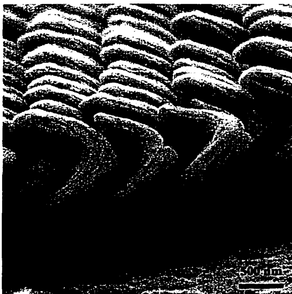
Figure 6.2 Scanning electron micrograph of regular array of large silicon helices with repeat distance a = 1250 nm. The film was deposited at angle of incidence \theta = 83^\circ deposition rate R = 30 \text{ \AA/s} and substrate rotation rate 0.1 \text{ min}^{-1} . The scale bar corresponds to 500 nm.
