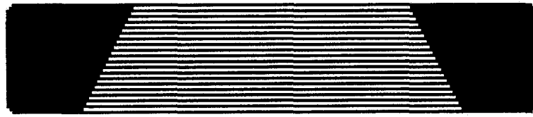
Figure 4-8: A crack propagation gage with twenty strands
