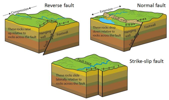
Figure 10.3.3: Depiction of reverse, normal, and strike-slip faults. Reverse faults happen during compression while normal faults happen during extension. Most strike-slip faults are related to transform boundaries.
