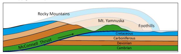
Figure 10.3.8: Depiction of the McConnell Thrust in the eastern part of the Rockies. The rock within the faded area has been eroded
