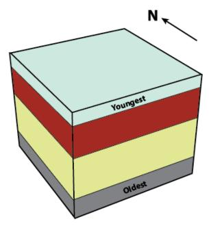
Figure 9.1.1: Block diagram of horizontal strata showing four distinct planar layers.
