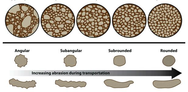
Figure C: A visual reference for descriptions of sorting (top) and roundness (bottom) of sediments and grains in clastic sedimentary rocks.
