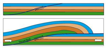
Figure 10.3.7: Depiction a thrust fault. Top: prior to faulting. Bottom: after significant fault offset.
