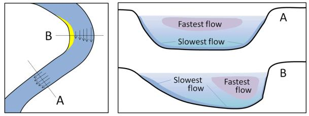
Figure 8.1.1: The relative velocity of stream flow depending on whether the stream channel is straight or curved (left), and with respect to the water depth (right). [Image Description]
