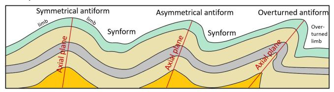
Figure 10.2.1: Examples of different types of folds and fold nomenclature. Axial planes are only shown for the anticlines, but synclines also have axial planes.
