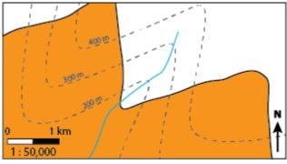
Figure 9.3.1: Use the Rule of V's to determine the dip direction of the two planar units (orange and white) shown on the map.
