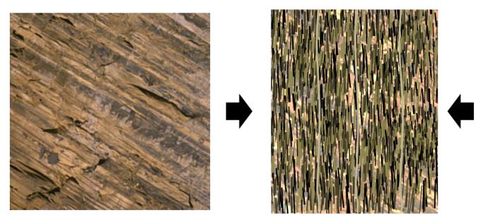
Figure 6.2.2: The textural effects of squeezing and mineral growth during regional metamorphism. The left diagram is shale with bedding slanting down to the right. The right diagram represents schist (derived from that shale), with mica crystals orientated perpendicular to the main stress direction and the original bedding no longer easily visible.
