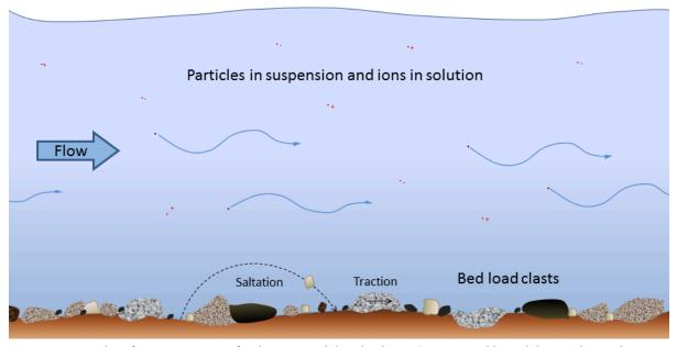
Figure 8.1.2: Modes of transportation of sediments and dissolved ions (represented by red dots with + and - signs) in a stream.
