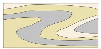
Figure 10.2.2: An isoclinal recumbent fold.
