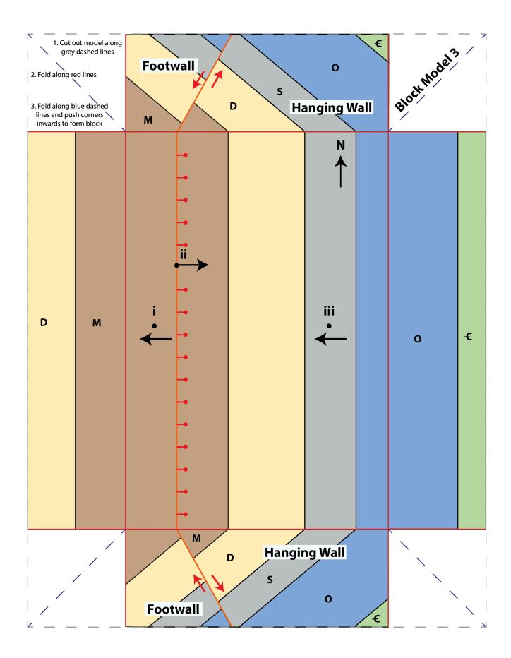
Reverse fault. Hanging wall has moved up relative to the footwall.
