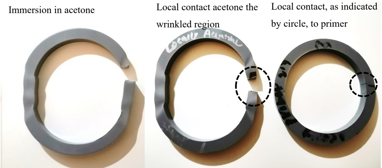
Figure 3-30 Presentation of CPVC ring specimens after D-split tests.
