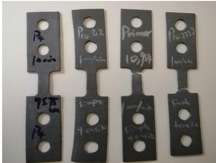
Figure 3-29 Presentation of primer-immersed CPVC dog-bone specimens in 'dry' test. The length of drying time is 96 hours, 312 hours, 984 hours and 2230 hours from left to right.
