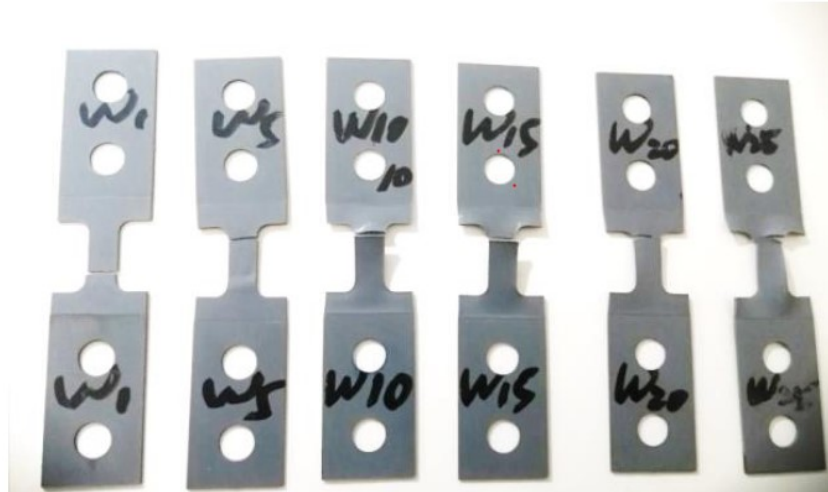
Figure 3-27 Presentation of acetone immersed CPVC dog-bone specimens in ‘wet’ tests. From left to right, the immersion time of specimen is 1, 5, 10, 15, 20 and 25 minute(s).
