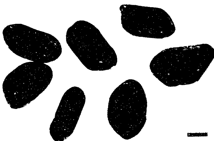
Figure 3.31 Two zircon populations from type-Nûk gneiss G87-149 a) anhedral, fractured, pink 'core' zircons b) euhedral, equant, high-U dark metamorphic zircons (oblique lighting, scale 100 \mu\text{m} ).
