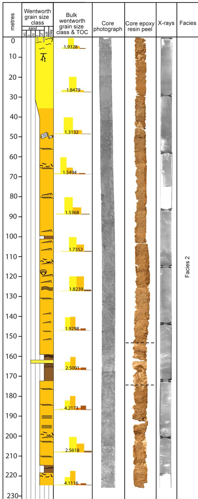
Fig. B-2: Vibracore 1 – Lois Island.
