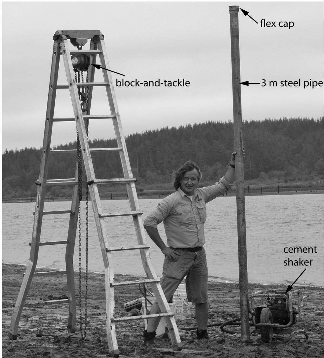
**Fig. 3-2:** Example of the vibracoring set-up used in this study.
