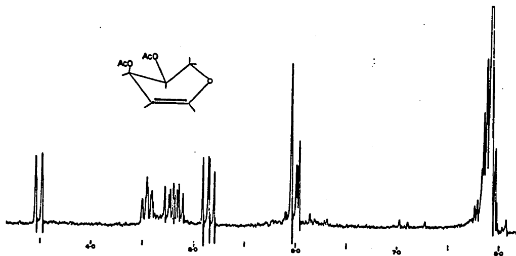
FIG. 12. N.m.r. spectrum (100 MHz) of di-O-acetyl-1,2-dideoxy-L- erythro -pent-1-enopyranose (XXVIII) (deuteriochloroform)
