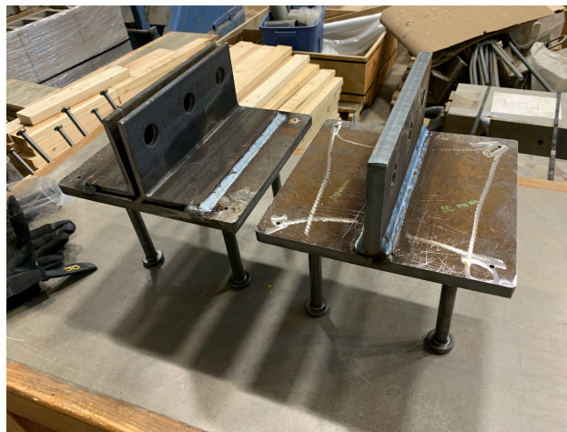
Figure 1.1 – Typical four-stud embedded plate with a double angle shear connection (left) and a shear tab (right) for connecting to the web of a wide-flange beam or channel.
