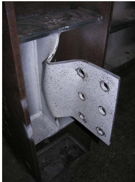
Figure 5-2: Out-of-plane deformation of specimen 3B-10-S-200C
