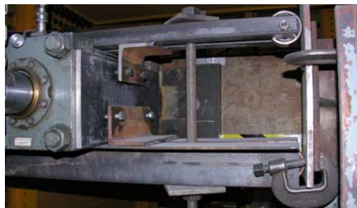
Figure 3-4: Actuator 3 lateral bracing system
