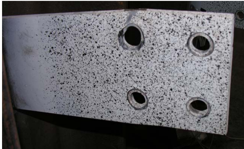
Figure 4-4: Plate deformation in specimen 2B-10-U-0
