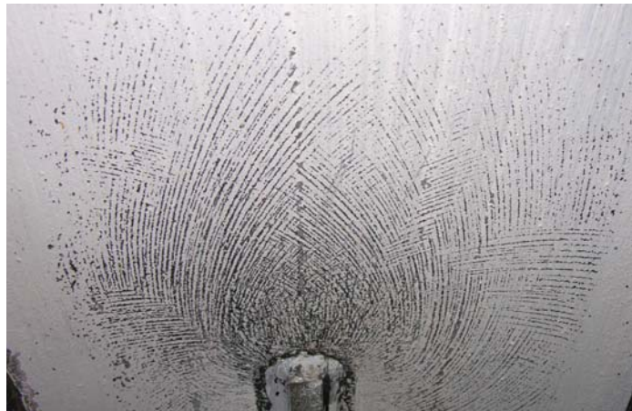
Figure 4-3: Lüders' lines at the compression edge of plate
