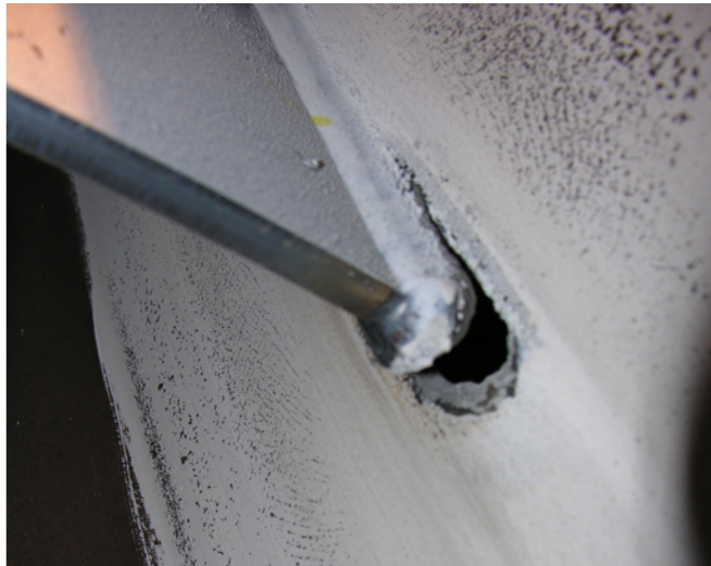
Figure 4-2: Column web tearing in specimen 5B-10-U-0
