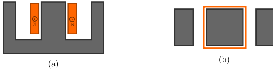
Figure 2.7: Incomplete inside window (IW) winding (a) Side View (b) Top View
