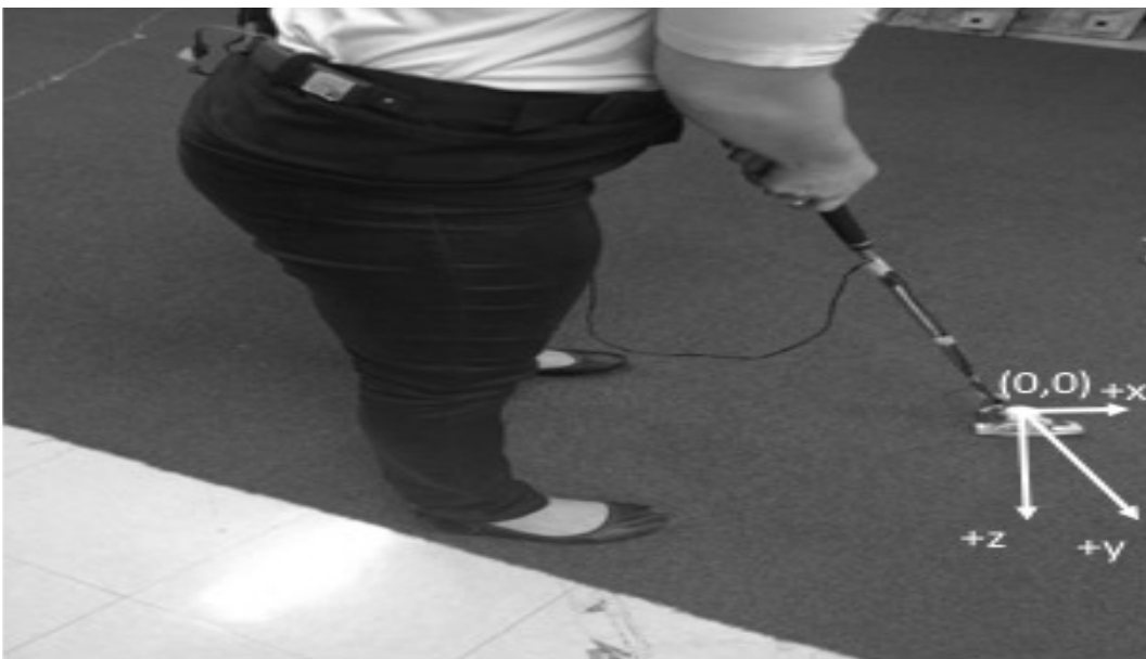
Figure 2.1. The environment was set up such that the flooring surface was along the XY plane and all putts were made along the negative Y axis while the +Z axis pointed into the floor. All balls started at the origin (0,0). Cameras were positioned on the ceiling on either corner of the surface (top image). Wired markers attached to the putter are plugged into a device that is plugged into a battery. These devices are worn on a belt and clipped around the participant's waist (bottom image).
