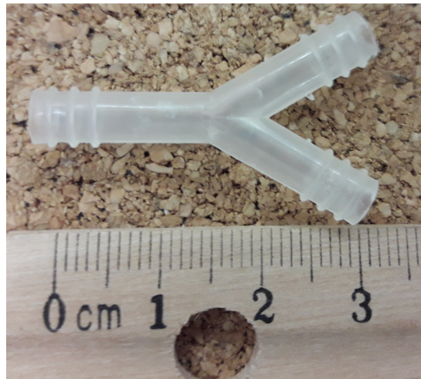
Figure A1.1: Y Polypropylene Connector (~0.5 cm diameter) used in y-maze, i.e. preference, experiments with ruler for scale. Flies were placed in the bent arms (right side of figure), and a mite was placed in the straight arm (left side of figure). Y-maze is displayed horizontal, as it was orientated during assays.
