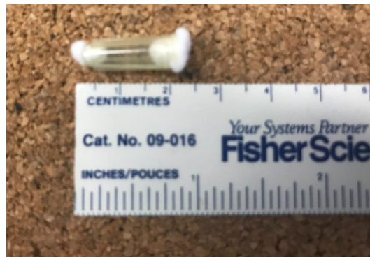
Figure A1.2: Cropped pipette tip (~0.5 cm internal diameter) used as a micro-arena. Individual flies were exposed to mite(s) either in the dark or the light. Following the exposure period, the number/presence of mite infections was recorded.
