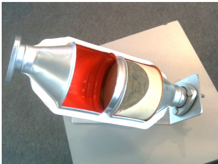
Figure 1.1: Picture of a catalytic converter showing the casing and the monolith. 1
