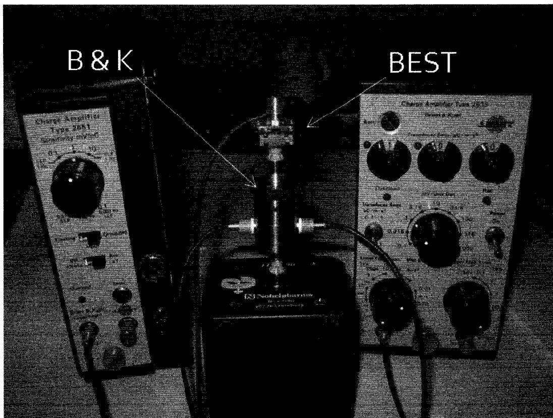
Figure 2-7. BEST transducer in series with a B & K impedance head connected to a TU-1000 skull simulator. Measures were not taken in this manner. The setup was displayed this way so that all equipment could fit easily in one Figure.
