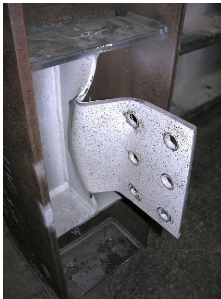
Figure 2-1: Out-of-plane deformation (Thomas et al. 2014)
