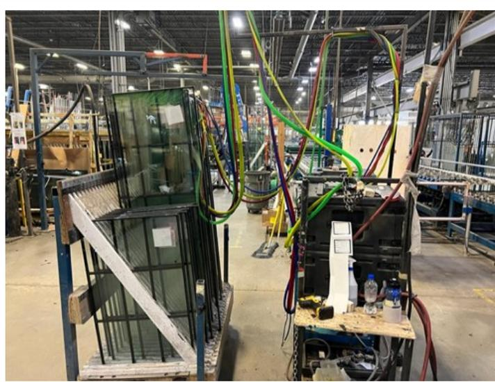
**Patching the Glass:** After filling the argon, workers use a patching gun to apply a sealant corner where the hole was made. The patching gun is a tool that allows for precise application of the sealant. They carefully dispense the sealant on the drilled hole. Once the patching is complete, the workers move on to smoothing the sealant on the corner of the glass where they spread the sealant, making it even and consistent across the surface.
