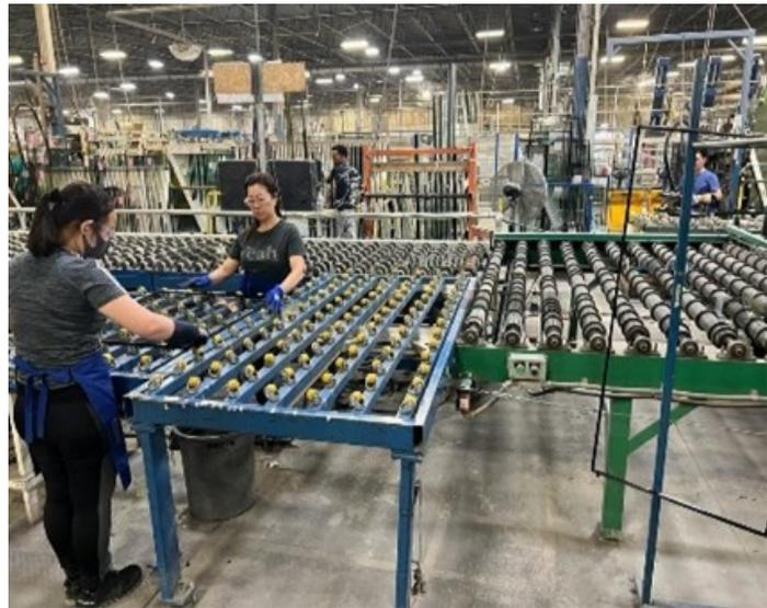
**Combining:** The two pieces of glass are then transported to a combining machine by conveyor and are combined via butterfly table.
