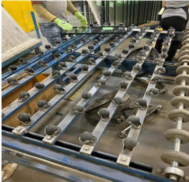
**Loading:** The glass units are loaded into carts and, once a cart reaches a capacity of 50 units, it is transported to the filling and argon station.
