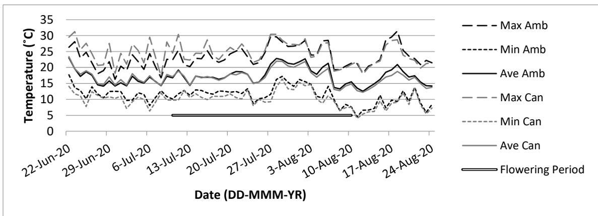
**Figure A. 38** Temperature in field 2 (F2), near Radway, AB, 2020. The average (Ave) daily temperature ( $^{\circ}\text{C}$ ), maximum (Max) and minimum (Min) values were measured under the canopy (Can) and above the crop canopy (Amb) with two HOBO U23-002 Temperature and Relative Humidity units.
