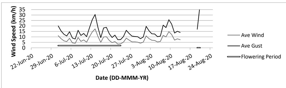
**Figure A. 58** Wind speed in field 5 (F5), near Legal, AB, 2020. Wind (km/h) was measured with a HOBO Davis Wind Speed and Direction Smart Sensor (S-WCF-M003).
