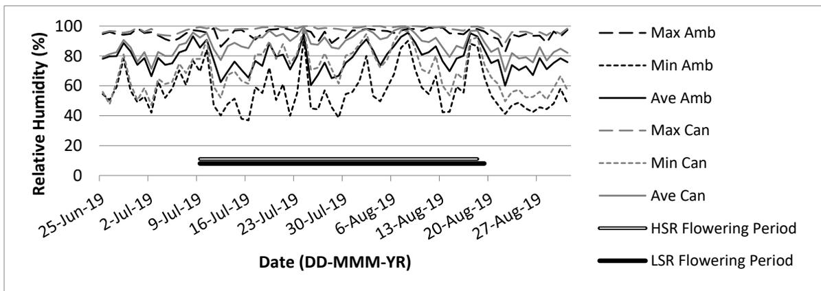
**Figure A. 24** Relative humidity (RH) near Beaverlodge, AB, 2019. The average (Ave) daily RH (%), maximum (Max) and minimum (Min) values were measured under the canopy (Can) and above the crop canopy (Amb) with two HOBO U23-002 Temperature and Relative Humidity units. The different seeding rate treatments and their corresponding flowering dates are represented as HSR (High seeding rate) and LSR (Low seeding rate).
