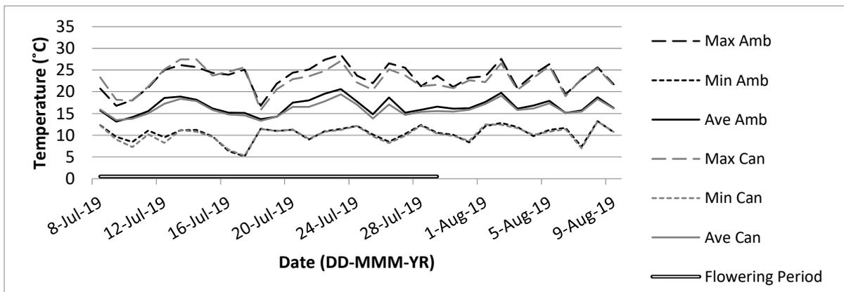
**Figure A. 34** Temperature in field 1 (F1) near Oliver, AB, 2019. The average (Ave) daily temperature (°C), maximum (Max) and minimum (Min) values were measured under the canopy (Can) and above the crop canopy (Amb) with two HOBO U23-002 Temperature and Relative Humidity units.
