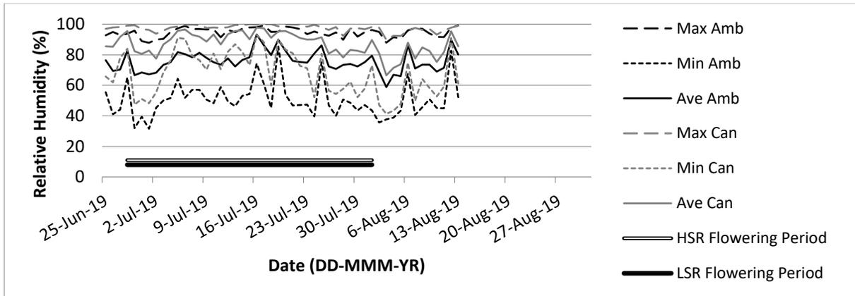
**Figure A. 27** Relative humidity (RH) near Outlook, SK, 2019. The average (Ave) daily RH (%), maximum (Max) and minimum (Min) values were measured under the canopy (Can) and above the crop canopy (Amb) with two HOBO U23-002 Temperature and Relative Humidity units. The different seeding rate treatments and their corresponding flowering dates are represented as HSR (High seeding rate) and LSR (Low seeding rate).
