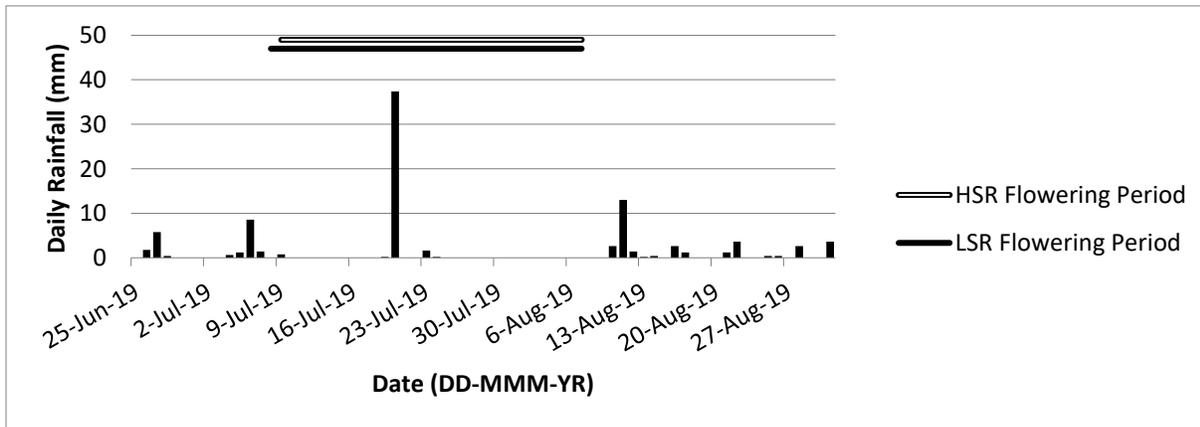
**Figure A. 14** Daily rainfall near Lethbridge, AB, 2019. Rain (mm) was measured with a HOBO Bucket Rain Gauge (RG3 – M). The different seeding rate treatments and their corresponding flowering dates are represented as HSR (High seeding rate) and LSR (Low seeding rate).
