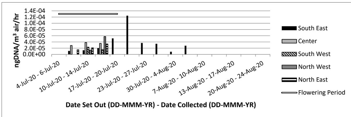
**Figure A. 106** Rotorod spore samples for 5 locations in field 4 (F4), near Legal, AB, 2020. *Sclerotinia sclerotiorum* airborne ascospores were captured by a GRIPST – 2009 Rotation Impact sampler (ngDNA/m<sup>3</sup>air/h) set at a 10% duty cycle placed in the field near the Spornado. Rods and cassettes were changed out twice per week during the canola flowering period.
