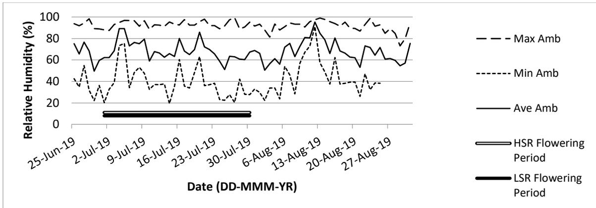
**Figure A. 29** Relative humidity (RH) near Brooks, AB, 2019. The average (Ave) daily RH (%), maximum (Max) and minimum (Min) values were measured above the crop canopy (Amb) with a HOBO U23-002 Temperature and Relative Humidity unit. The different seeding rate treatments and their corresponding flowering dates are represented as HSR (High seeding rate) and LSR (Low seeding rate).
