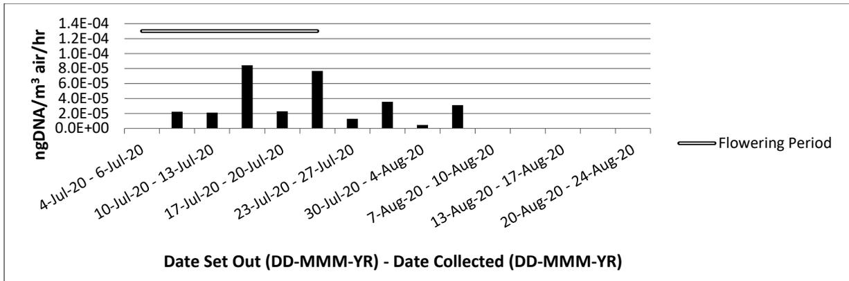
**Figure A. 89** *Sclerotinia sclerotiorum* airborne ascospores for Field 5 (F5), near Legal, AB, 2020 were captured by a GRIPST – 2009 Rotation Impact Sampler (ngDNA/m<sup>3</sup>air/h) set at a 10% duty cycle placed in the field near the Spornado. Rods were changed out twice per week during the canola flowering period.
