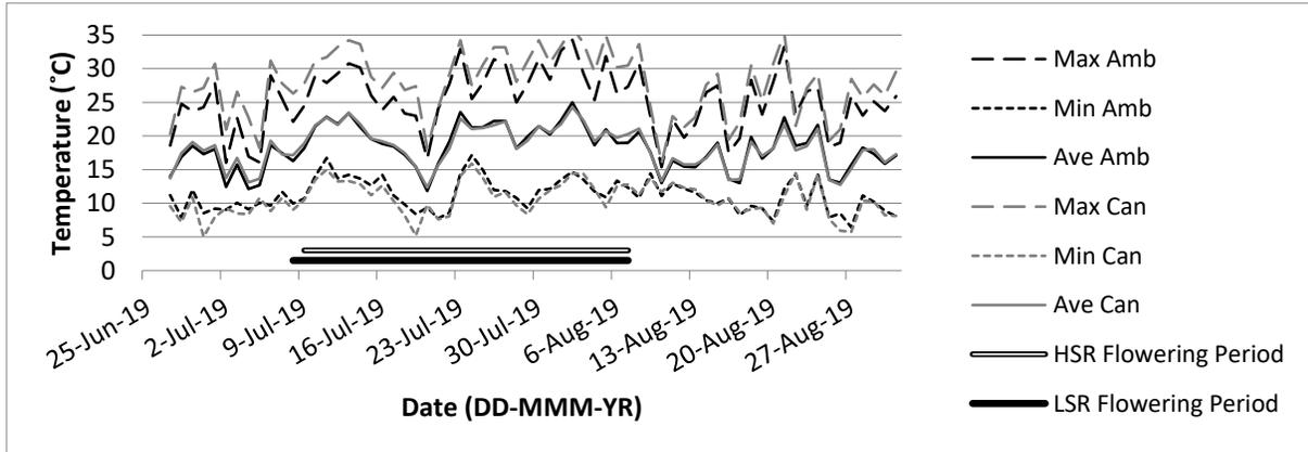
**Figure A. 44** Temperature near Lethbridge, AB, 2019. The average (Ave) daily temperature ( $^{\circ}\text{C}$ ), maximum (Max) and minimum (Min) values were measured under the canopy (Can) and above the crop canopy (Amb) with two HOBO U23-002 Temperature and Relative Humidity units. The different seeding rate treatments and their corresponding flowering dates are represented as HSR (High seeding rate) and LSR (Low seeding rate).
