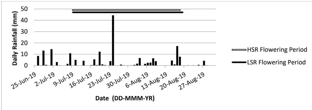
**Figure A. 13** Daily rainfall near Beaverlodge, AB, 2019. Rain (mm) was measured with a HOBO Bucket Rain Gauge (RG3 – M). The different seeding rate treatments and their corresponding flowering dates are represented as HSR (High seeding rate) and LSR (Low seeding rate).
