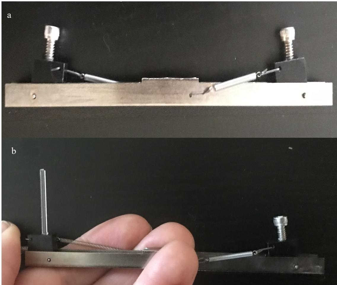
**Figure 3.2** GRIPST-2009 Rotation Impaction Sampler (rotorod) used to monitor *Sclerotinia sclerotiorum* ascospore levels in this study. Close up of a) sampling head at rest with rods retracted and b) sampling head with a single silicone covered rod exposed.
