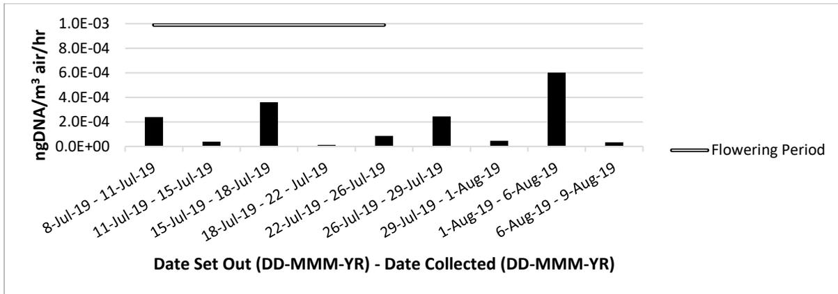
**Figure A. 83** *Sclerotinia sclerotiorum* airborne ascospores for Field 2 (F2), near Namao, AB, 2019 were captured by a GRIPST – 2009 Rotation Impact Sampler (ngDNA/m<sup>3</sup>air/h) set at a 10% duty cycle placed in the field near the Spornado. Rods were changed out twice per week during the canola flowering period.
