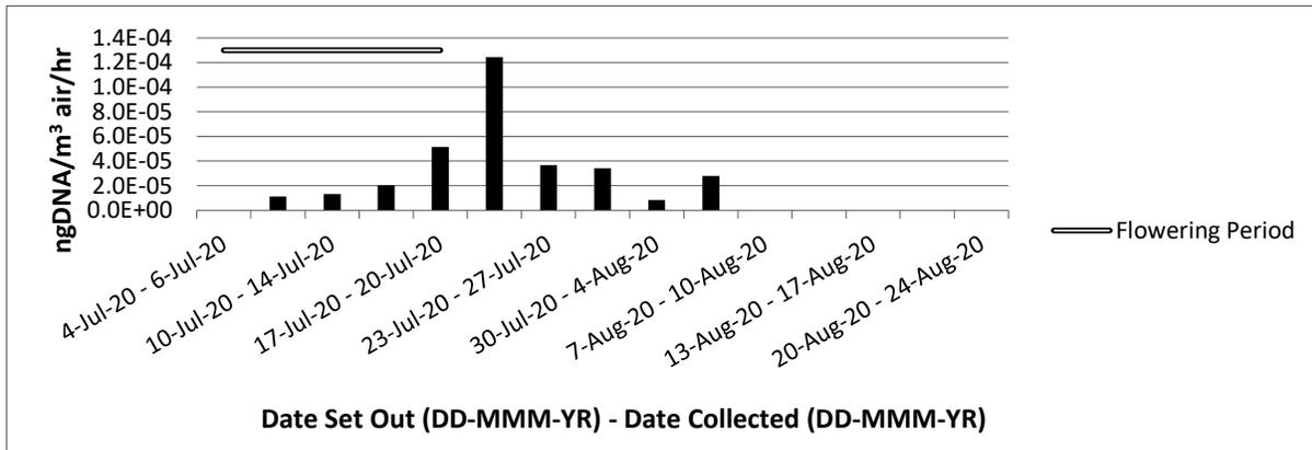
**Figure A. 88** *Sclerotinia sclerotiorum* airborne ascospores for Field 4 (F4), near Legal, AB, 2020 were captured by a GRIPST – 2009 Rotation Impact Sampler (ngDNA/m<sup>3</sup>air/h) set at a 10% duty cycle placed in the field near the Spornado. Rods were changed out twice per week during the canola flowering period.
