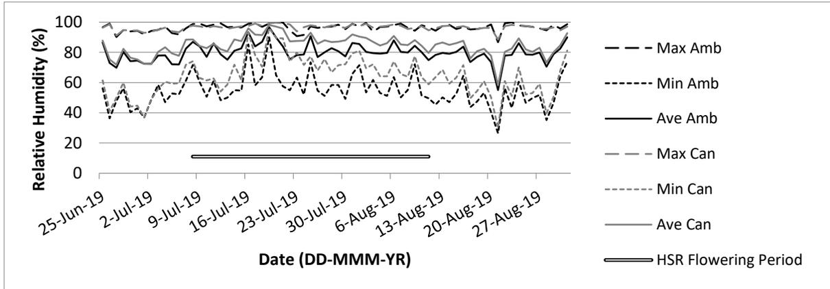
**Figure A. 28** Relative humidity (RH) near Scott, AB, 2019. The average (Ave) daily RH (%), maximum (Max) and minimum (Min) values were measured under the canopy (Can) and above the crop canopy (Amb) with two HOBO U23-002 Temperature and Relative Humidity units. The different seeding rate treatments and their corresponding flowering dates are represented as HSR (High seeding rate) and LSR (Low seeding rate), although no flowering dates were recorded the lower seeding rate for Scott, AB.
