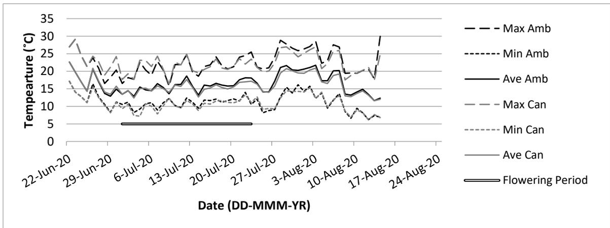
**Figure A. 42** Temperature in field 5 (F5), near Legal, AB, 2020. The average (Ave) daily temperature ( $^{\circ}\text{C}$ ), maximum (Max) and minimum (Min) values were measured under the canopy (Can) and above the crop canopy (Amb) with two HOBO U23-002 Temperature and Relative Humidity units.
