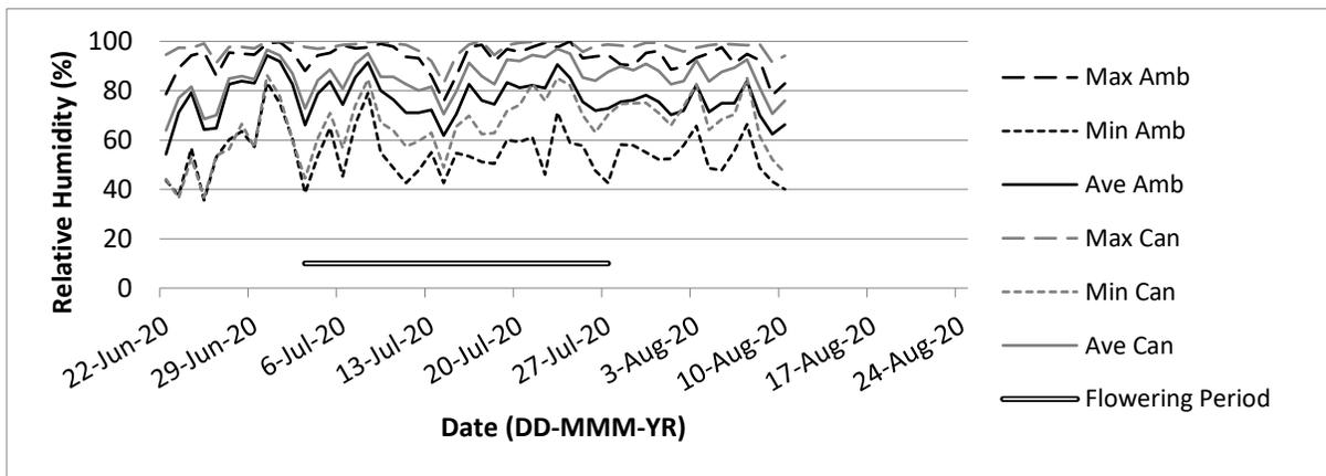
**Figure A. 20** Relative humidity (RH) in field 1 (F1), near Radway, AB, 2020. The average (Ave) daily RH (%), maximum (Max) and minimum (Min) values were measured under the canopy (Can) and above the crop canopy (Amb) with two HOBO U23-002 Temperature and Relative Humidity units.
