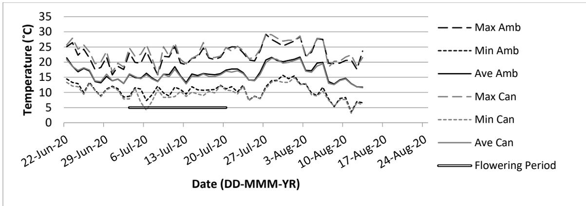
**Figure A. 41** Temperature in field 4 (F4), near Legal, AB, 2020. The average (Ave) daily temperature ( $^{\circ}\text{C}$ ), maximum (Max) and minimum (Min) values were measured under the canopy (Can) and above the crop canopy (Amb) with two HOBO U23-002 Temperature and Relative Humidity units.
