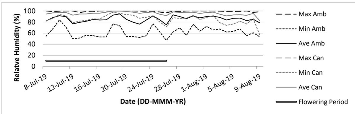
**Figure A. 16** Relative humidity (RH) in field 2 (F2), near Namao, AB, 2019. The average (Ave) daily RH (%), maximum (Max) and minimum (Min) values were measured under the canopy (Can) and above the crop canopy (Amb) with two HOBO U23-002 Temperature and Relative Humidity units.
