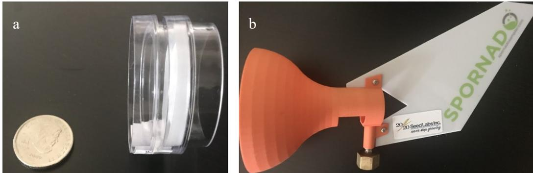
**Figure 3.1.** Spornado passive spore trap used to monitor *Sclerotinia sclerotiorum* ascospore levels in this study. a) Spornado cassette and b) Spornado. Cassettes were switched every 3-4 days from just before flowering until flowering had completed.
