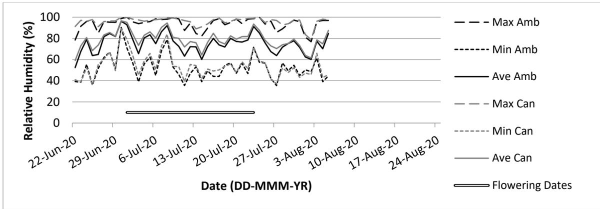
**Figure A. 19** Relative humidity (RH) in field 3 (F3), near Oliver, AB, 2020. The average (Ave) daily RH (%), maximum (Max) and minimum (Min) values were measured under the canopy (Can) and above the crop canopy (Amb) with two HOBO U23-002 Temperature and Relative Humidity units.
