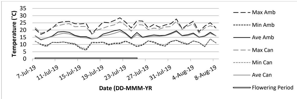
**Figure A. 35** Temperature in field 4 (F4), near Oliver, AB, 2019. The average (Ave) daily temperature ( $^{\circ}\text{C}$ ), maximum (Max) and minimum (Min) values were measured under the canopy (Can) and above the crop canopy (Amb) with two HOBO U23-002 Temperature and Relative Humidity units.
