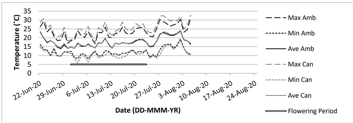
**Figure A. 40** Temperature in field 3 (F3), near Oliver, AB, 2020. The average (Ave) daily temperature ( $^{\circ}\text{C}$ ), maximum (Max) and minimum (Min) values were measured under the canopy (Can) and above the crop canopy (Amb) with two HOBO U23-002 Temperature and Relative Humidity units.
