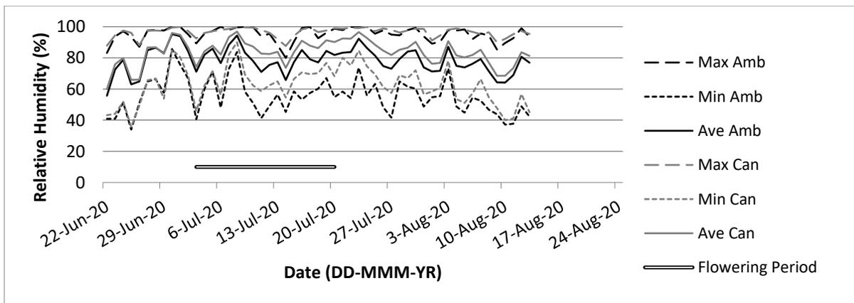
**Figure A. 22** Relative humidity (RH) in field 4 (F4), near Legal, AB, 2020. The average (Ave) daily RH (%), maximum (Max) and minimum (Min) values were measured under the canopy (Can) and above the crop canopy (Amb) with two HOBO U23-002 Temperature and Relative Humidity units.
