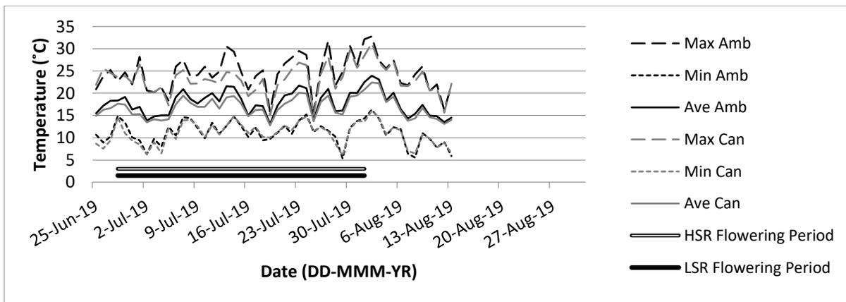
Figure A. 50 Temperature near Outlook, SK, 2019. The average (Ave) daily temperature ( $^{\circ}\text{C}$ ), maximum (Max) and minimum (Min) values were measured under the canopy (Can) and above the crop canopy (Amb) with two HOBO U23-002 Temperature and Relative Humidity units. The different seeding rate treatments and their corresponding flowering dates are represented as HSR (High seeding rate) and LSR (Low seeding rate).
