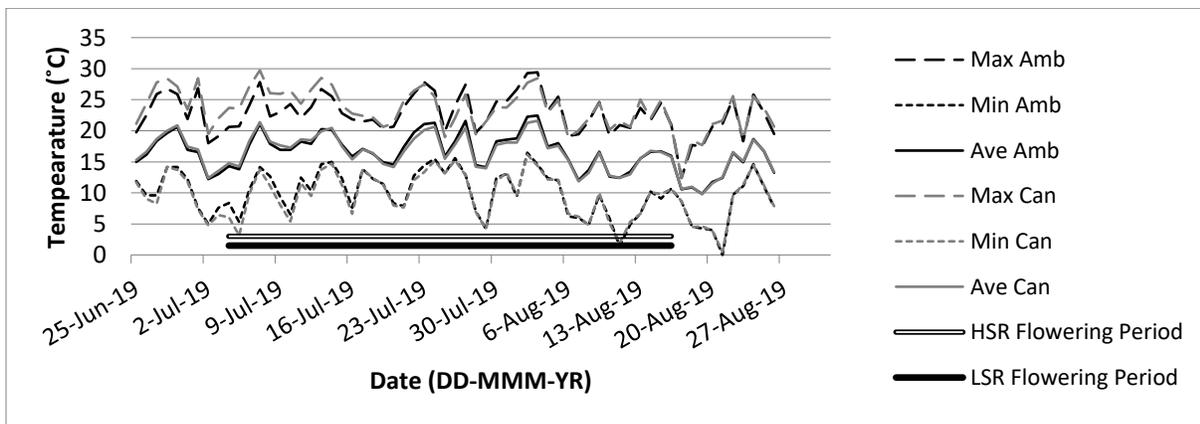
**Figure A. 52** Temperature near Normandin, QC, 2019. The average (Ave) daily temperature ( $^{\circ}\text{C}$ ), maximum (Max) and minimum (Min) values were measured under the canopy (Can) and above the crop canopy (Amb) with two HOBO U23-002 Temperature and Relative Humidity units. The different seeding rate treatments and their corresponding flowering dates are represented as HSR (High seeding rate) and LSR (Low seeding rate).
