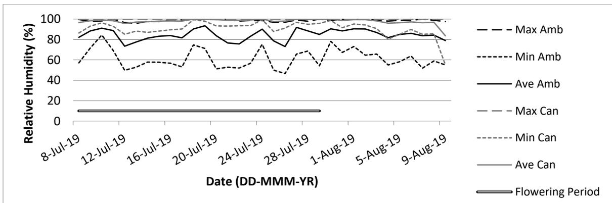
**Figure A. 18** Relative humidity (RH) in field 4 (F4), near Oliver, AB, 2019. The average (Ave) daily RH (%), maximum (Max) and minimum (Min) values were measured under the canopy (Can) and above the crop canopy (Amb) with two HOBO U23-002 Temperature and Relative Humidity units.
