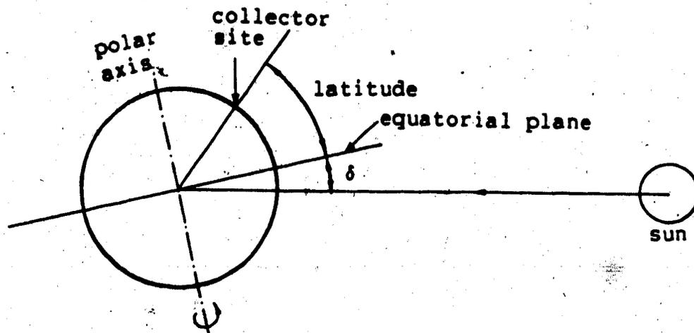
Figure 3.1. Solar declination (adapted from ASHRAE, 1971)
