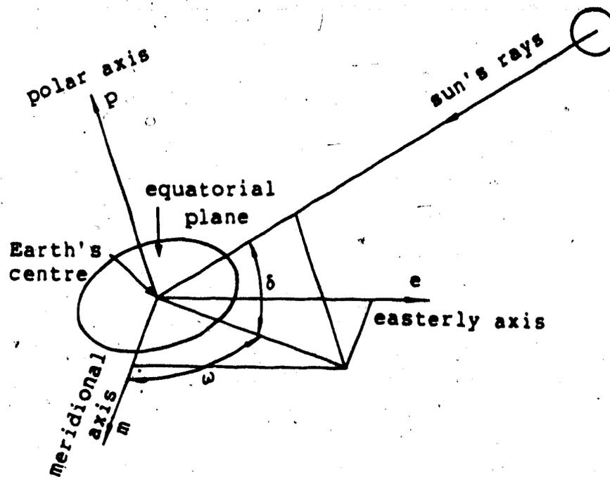
Figure 3.3 Hour angle (adapted from ASHRAE, 1971)
