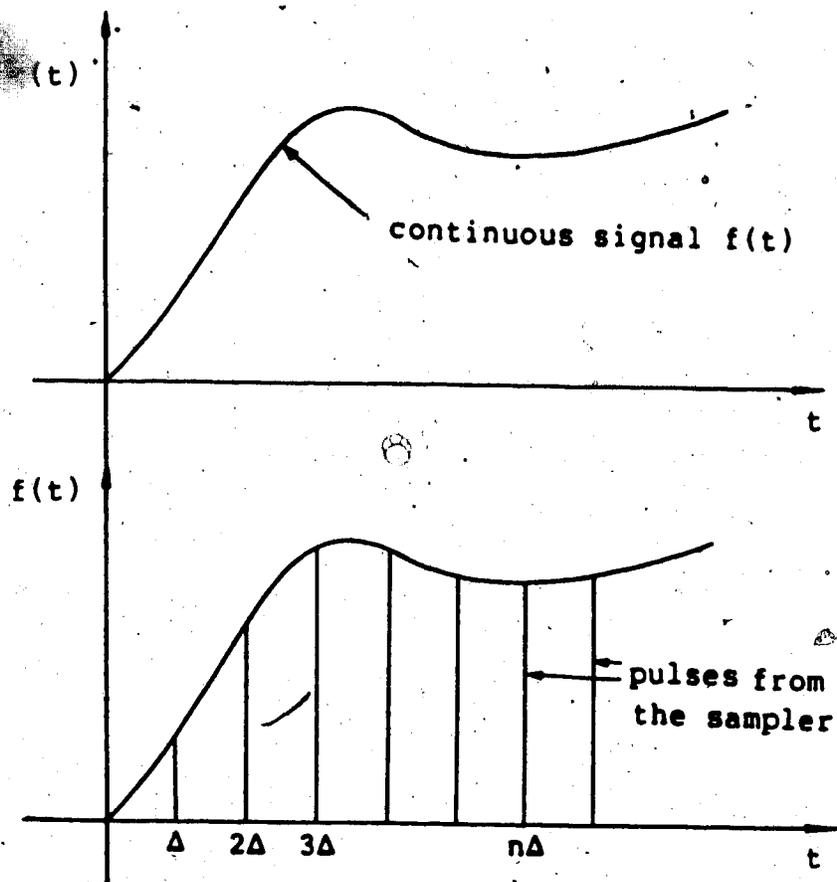
Figure 2.3 Pulses output from a sampler of a continuous function
