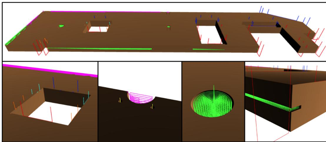
Figure 4-20. 3D plot of CLT panel with paths generated by the algorithm TPPA. The color code of the lines represents different operations and robots. The color code for robot 1 is green for end mill, aqua green for drilling, orange for the circular saw of 10 inches, and red for circular saw of 500 millimeters. Color code for robot 2, pink for end mill, yellow for drilling, light blue for the circular saw of 10 inches, and blue for circular saw of 500 millimeters.
