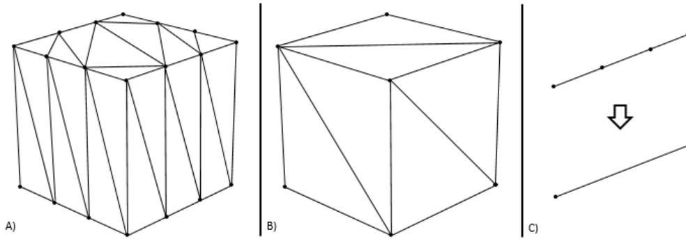
Figure 4-12. Example of simple geometry with overcrowded mesh. A) Simple cube with excessive mesh points, B) cube with simplified mesh, and C) example of multiple segments optimized to single line.
