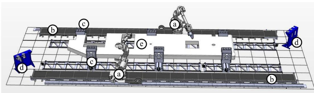
Figure 4-19. Automated robotic machining cell for cross-laminated timber panels: (a) Robot ABB® IRB 7600; (b) Track motion ABB® IRBT 7004; (c) Flexible clamping System; (d) Tool stand; (e) CLT Panel for reference.
