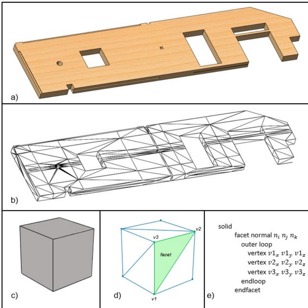
Figure 4-5. Standard Triangle Language “STL” format visualization. a) 3D model representation of CLT panel on BIM/CAD format, b) STL representation of the same CLT panel, c) Common 3D model of a cube seen on BIM/CAD format, d) STL model of the same cube showing the vertices of one triangle and its facet, e) format structure for the ASCII STL showing the framework of the vertices and facet.
