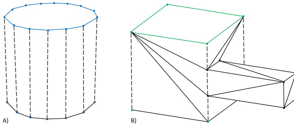
Figure 4-9. Projection of the top boundary on the bodies for the calculation of the depth. A) cylindrical object, and B) prismatic object.
