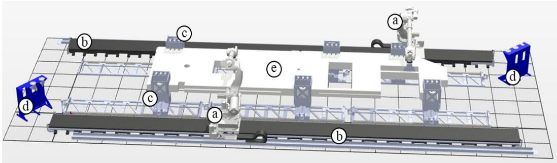
Figure 3-5. Automated robotic machining cell for cross-laminated timber panels: (a) Robot ABB® IRB 7600; (b) Track motion ABB® IRBT 7004; (c) Flexible clamping System; (d) Tool stand; (e) Minimum viable product.
