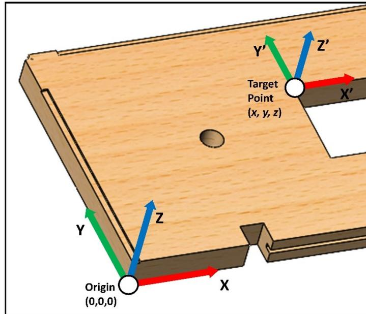
Figure 4-1. Example of target point for the coordinate system.
