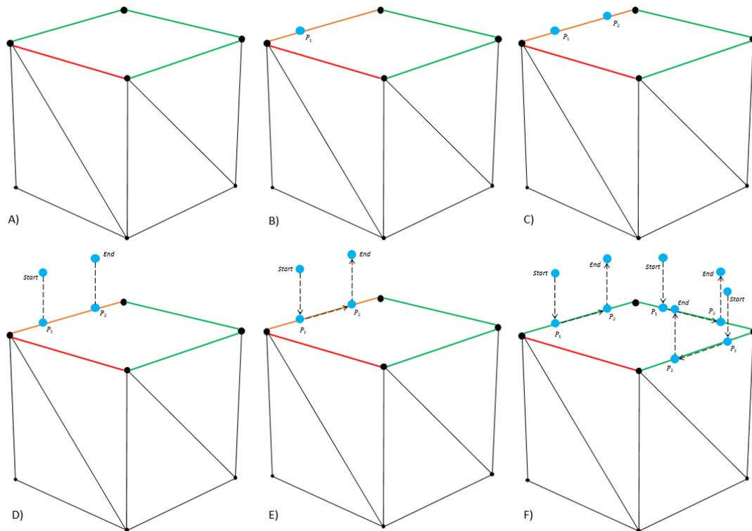
Figure 4-16. Sequence of sawing process for the top lines. A) identification of the external line highlighted in red, B) identification of the start point for one line, C) identification of the end point for one line, D) generation of the targets in a z offset for safety position of the robot, E) target path generated following the points created, and F) paths created on the rest of the remaining lines.
