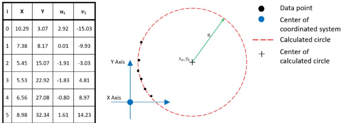
Figure 4-8. Example of Least-Square Circle fit method [162]. The left side table shows the data used for the example in coordinates (x,y) and (u,v). On the right side, a visualization is shown of the circle which fits to the points given and presents an idea of the center of the circle and its radius.
