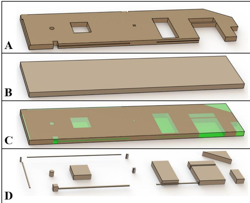
Figure 4-6. Boolean operation of the processed panel. a) original design, b) raw material required, c) overlapped model of raw material and desired design with the remaining material highlighted in green, d) bodies obtained from the boolean operation.
