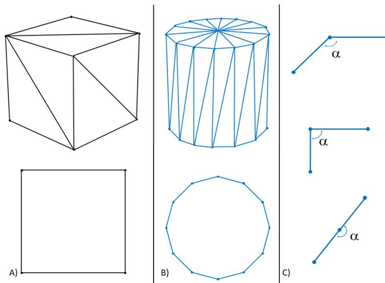
Figure 4-7. Top surface analysis of STL geometries. A) prismatic bodies representation and its top surface, B) cylindrical bodies representation and its top surface, and C) angles found in between edges of boundary (obtuse, right, or straight).
