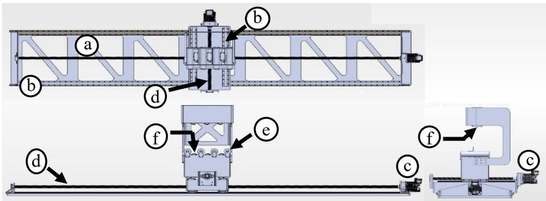
Figure 3-3. Flexible clamping station: (a) Steel plate; (b) Wide ball bearing carriage and rail; (c) Servomotor CPM-MCVC-D1003P-RLN; (d) Worm gear; (e) Industrial polymer rolls; (f) Pneumatic cylinder SMC HYG50TFR-200.
