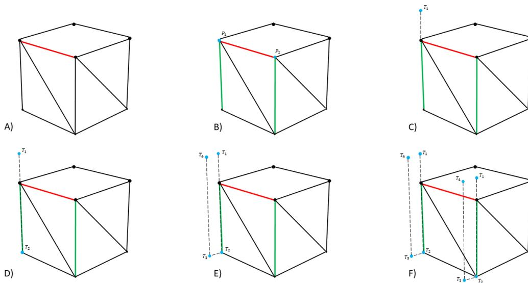
Figure 4-17. Sequence of sawing process of the side cuts required in external lines. A) identification of the external line highlighted in red, B) identification of the two end points of the external lines, C) generation of the first target in an  $z$  offset, D) second target generated in the bottom of the panel, E) third and the fourth target generated in a projection of opposite direction of the next line in the boundary, and F) target path for both reference points.
