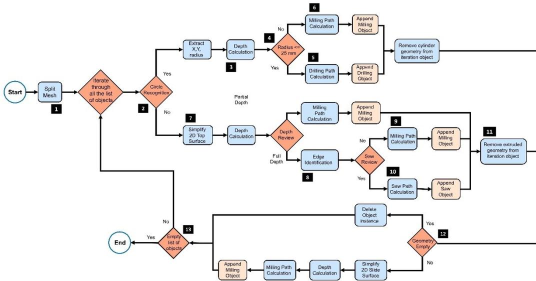
Figure 4-4. Overall algorithm for the target extraction of the cutting operations for the CLT panel.
