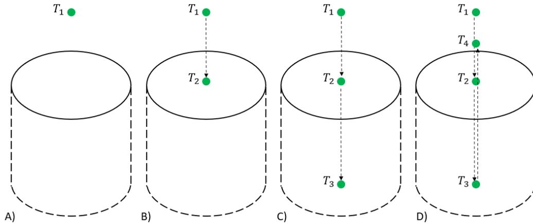
Figure 4-10. Sequence for the four targets required in the path of the drilling operation. A) first target with clearance for the robot, B) second target on the initial point of the drilling hole, C) target on the depth of the hole but limited to 90 mm, and D) target with enough clearance for the robot to switch to the next operation.
