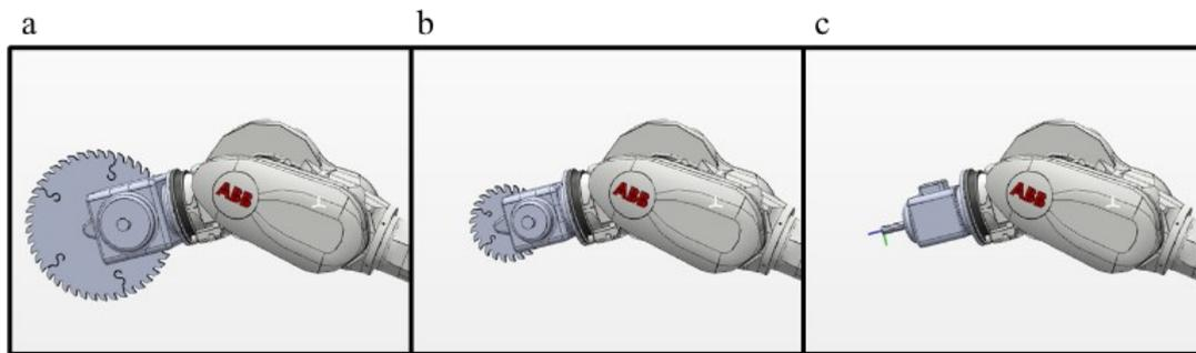
Figure 3-2. Tools design representation in RobotStudio®: (a) circular saw of 500 mm of diameter; (b) circular saw of 10 inches of diameter; and (c) rough end mill of 25 mm of diameter.
