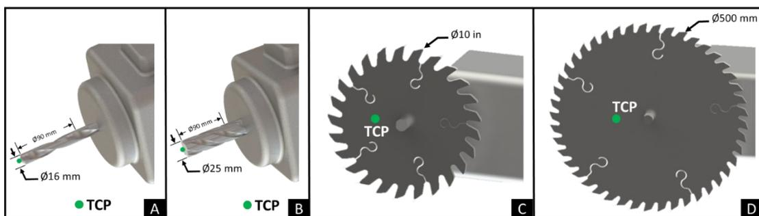
Figure 4-3. Tools considered in the algorithm. A) drill bit of 16 mm of diameter, B) end mill with 25 millimeters of diameter, C) circular saw with 10 inches of diameter, and D) circular saw with 500 millimeters of diameter.
