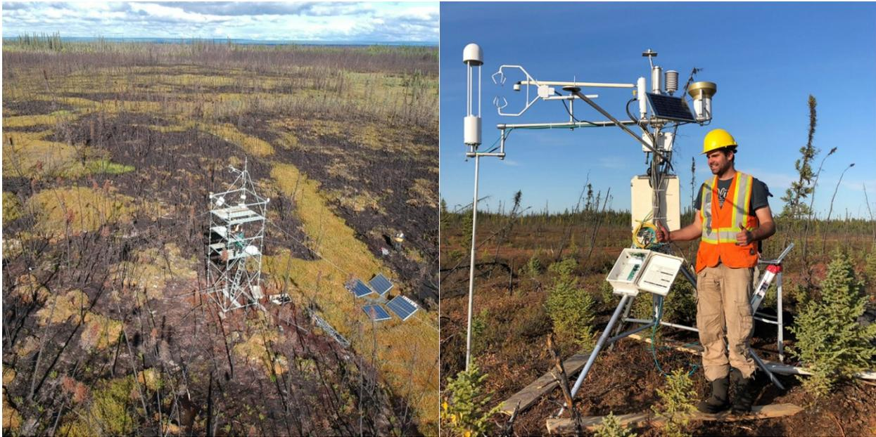
**Figure A4.1:** Images of eddy covariance tower setup. Left: scaffolding structure at the 2019 Burn to bring high-frequency instrumentation above the tree canopy. Right: tripod structure at 2007 Burn where most burned tree remainders have fallen to the ground and regrowth of vegetation is still below 1 meter in height.
