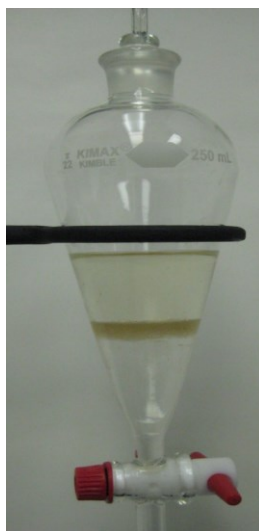
Figure 3.6. Extraction of acidified tailings water (0.5 wt.% NaOH) with DCM
