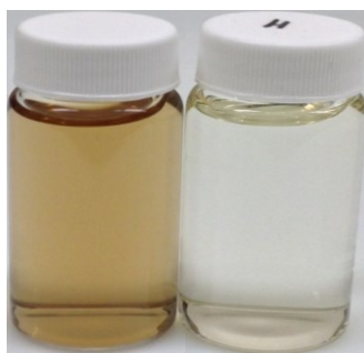
Figure C.3. Left: tailings water with 50 ppm humic acids, Right: tailings water with 50 ppm humic acids after being treated with illite clay.
