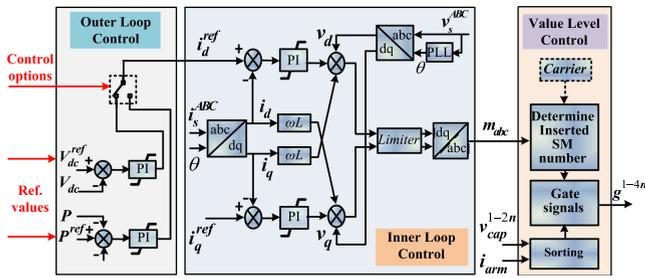
FIG. 4. The ICT-enabled PD-SPWM MMC control scheme.
