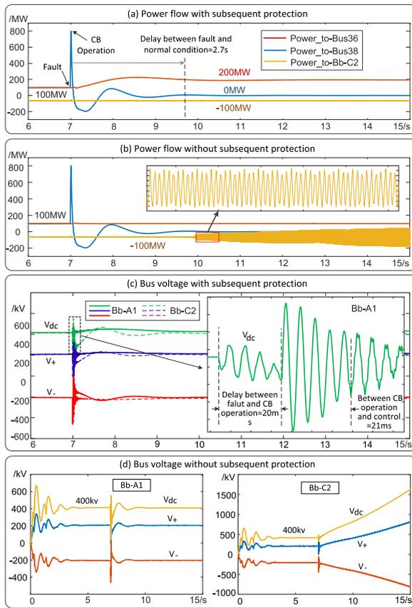
**FIG. 7. DC fault protection case: (a-b) power flowing to different buses with and without subsequent protection; (c-d) positive, negative pole voltage and DC voltage of converter Bb-A1 and Bb-C2 with and without subsequent protection.**
