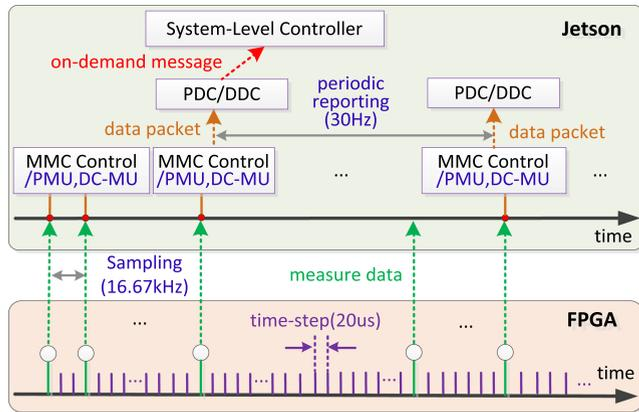
FIG. 5. Demonstration of interaction between power system emulation and communication network simulation.
