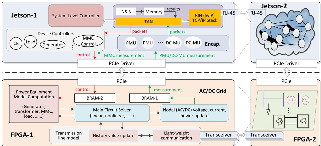
FIG. 2. Top level architecture of the heterogeneous co-emulation hardware architecture on the multiple Jetson-FPGA platform.
