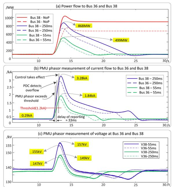
**FIG. 6. Power overflow case: (a) comparison of the power flowing to Bus36 and Bus38 with 55 ms, 250 ms response delay and without protection; (b-c) comparison of phasor magnitude of the current flowing to Bus36 and Bus38 and bus voltages with 55 ms and 250 ms response delay.**
