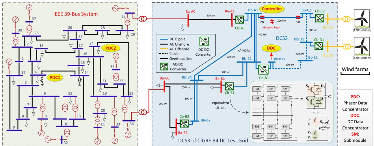
FIG. 1. Hybrid AC/DC test power system used in this work.
