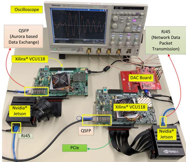
FIG. 3. Hardware setup for the heterogeneous co-emulator.
