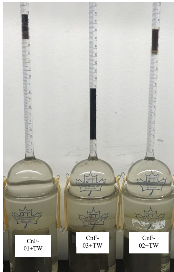
Figure 5.1: Core plugs in Amott cells, from left to right: CnF-01+TW, CnF-03+TW, and CnF-02+TW.
