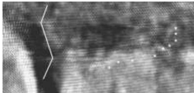
Figure 1. 12 An HREM image of a twin formed by plastically deforming electrodeposited NC Ni. The twin was formed by the emission of partials from the grain boundary on the left, and it ended in the grain interior as marked by the white asterisks [63].
