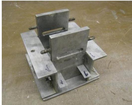
Figure A. 9. Mold used to make discontinuous synthetic rock with open crack.
