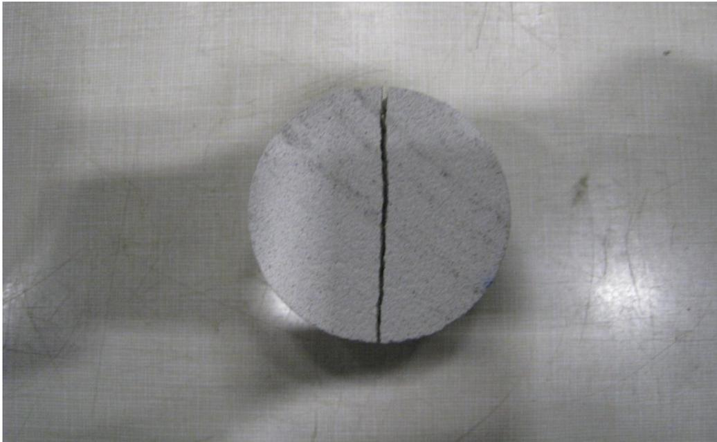
Figure 3.4. Tensile fracture of the sample after the Brazilian Test.
