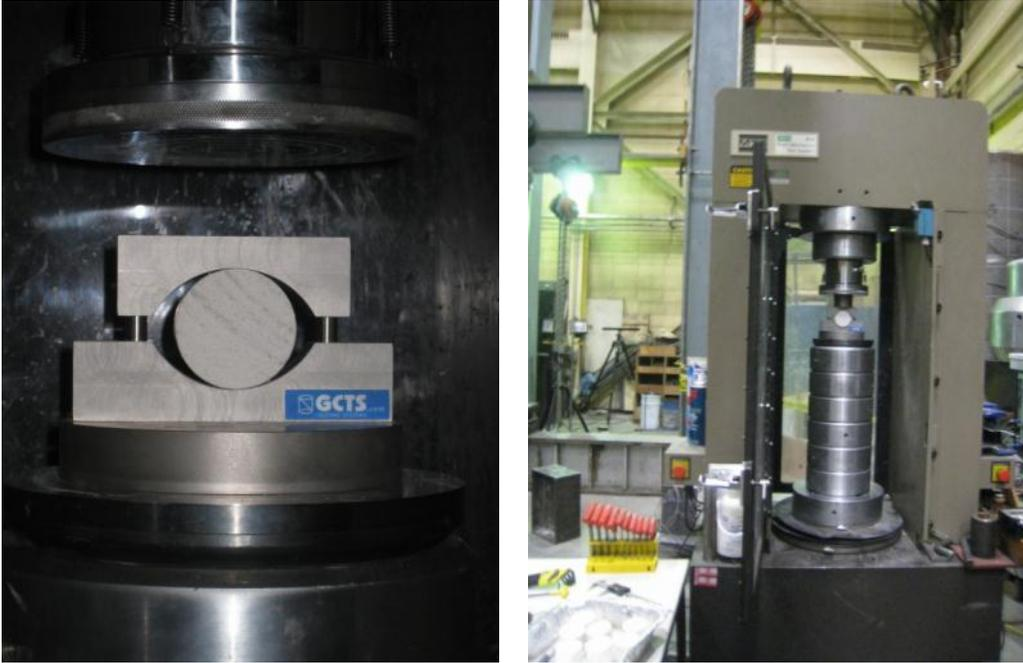
Figure A. 3. Loading plate and test system of the Brazilian Test.
