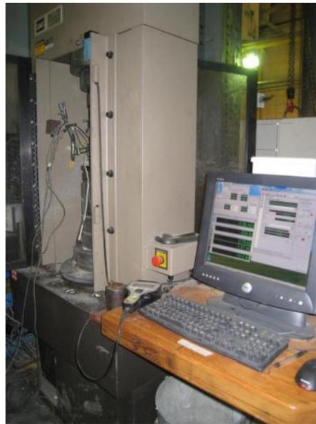
Figure A. 2 Data acquisition system connected to the rock mechanics testing system.
