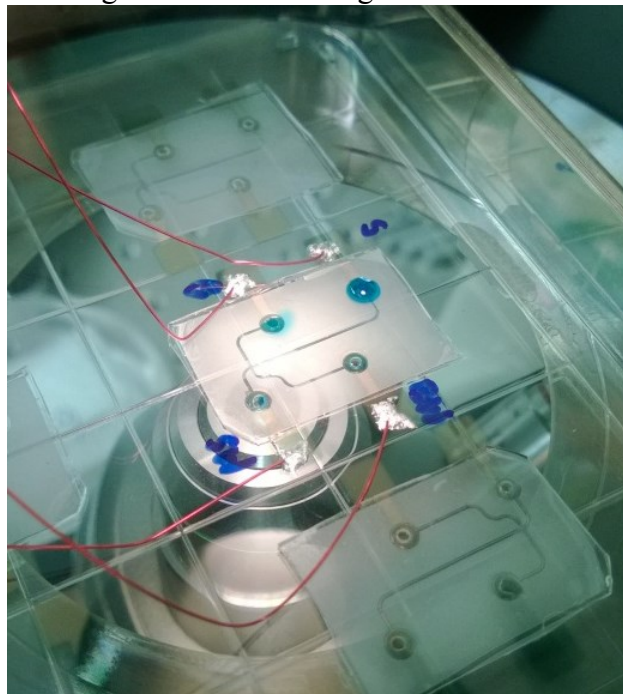
Fig D5: Assembled Microfluidic Chip on the soldered polymer substrate.
