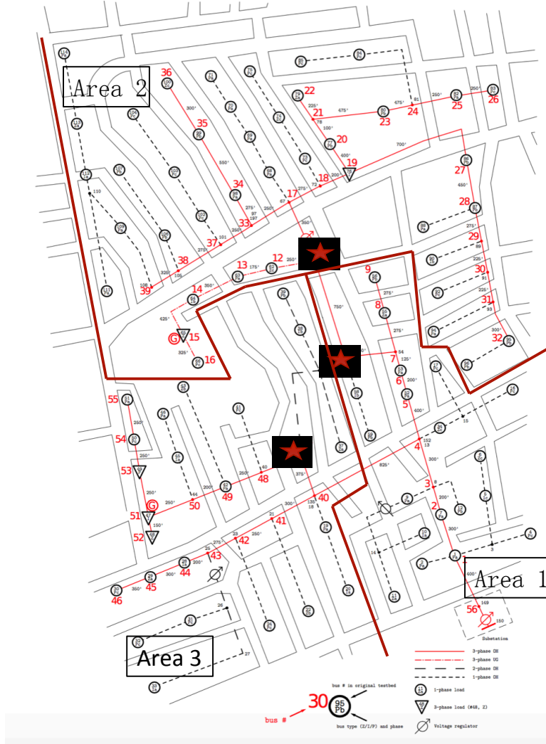
Figure 3.4: Topology of the Distribution System in Case Study.
