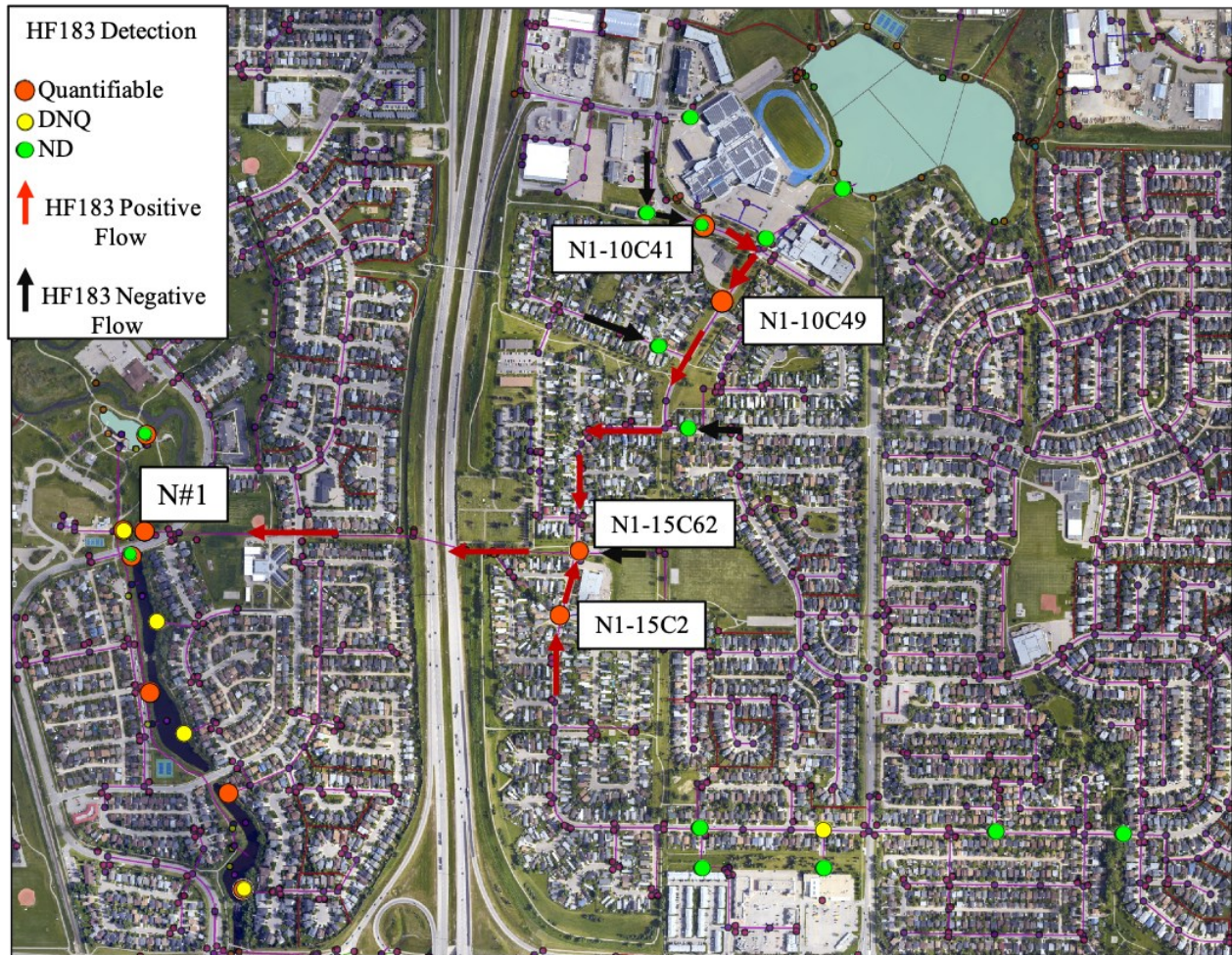
Figure 4-11. Map of Nose Creek stormwater drainage network summarizing the most relevant manholes tested for human sewage marker HF183 upstream of HF183 positive outfall site N#1. Note the manholes upstream of N#1 where HF183 was positive and quantifiable (red dots), detectable but not quantifiable (yellow dots), or not detected (green dots). Note also the flow of stormwater through the system, represented by presumed HF183 positive flow (red arrows) based on upstream site HF183 detection and concentrations, as well as flow with no demonstrable HF183 detection (black arrows).
