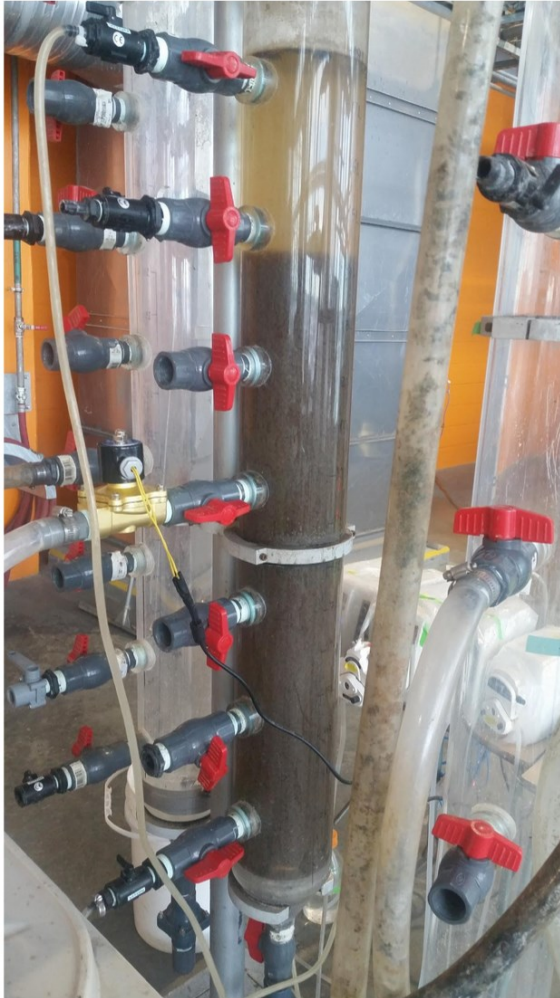
Figure 4-1. PR1 with added sludge during first stages of operation. The reactor was seeded with AS and nitrification/denitrification AGS from a lab-scale system.
