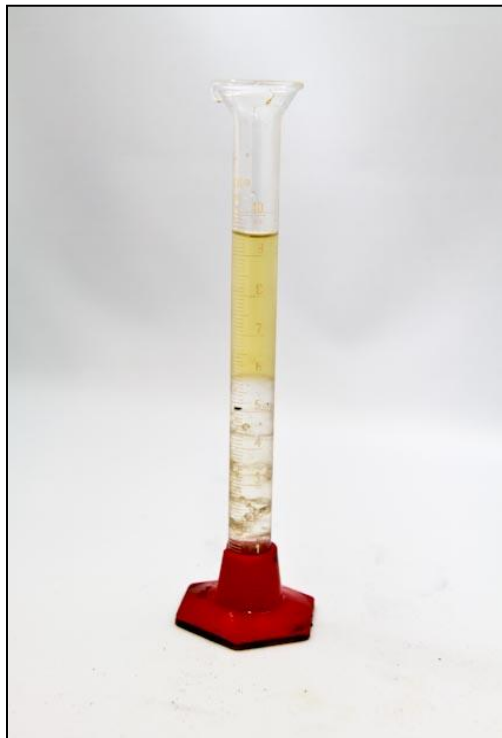
Figure 28: Solvent+oil production during Phase 3 for low injection rate, 0.15 cc/min (at initial stages).
