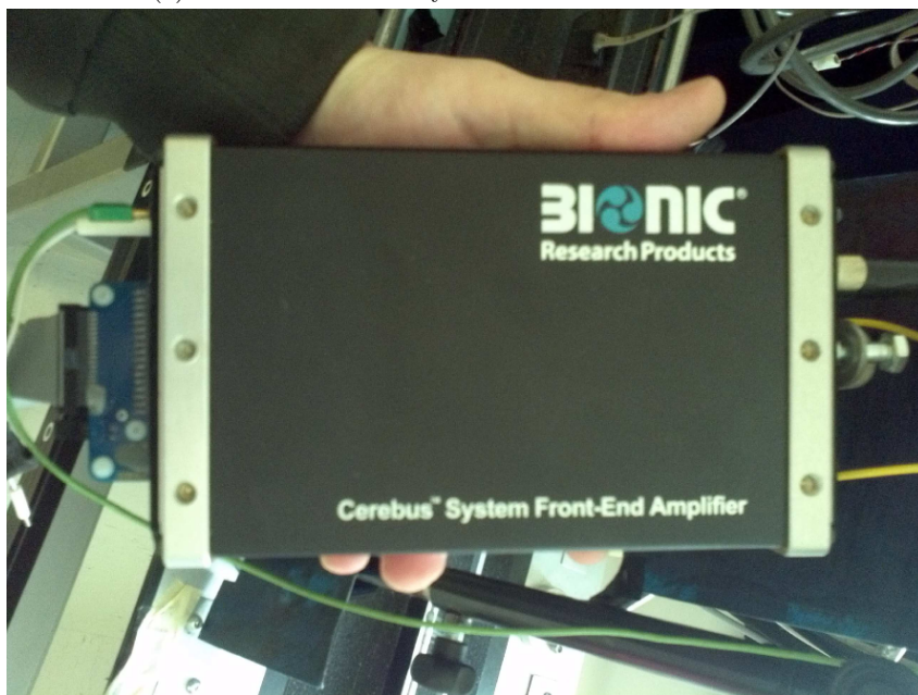
(b) Analog front-end with optical data transmission.
