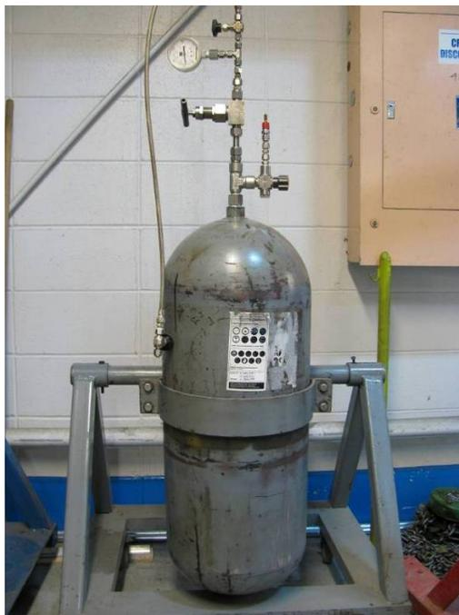
**FIGURE 3-26 60-L STEEL CYLINDRICAL CONTAINER USED TO SATURATE DRY BURNT LAKE BITUMEN WITH METHANE**
