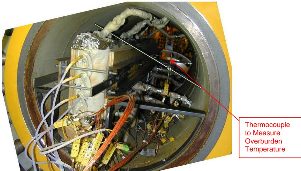
**FIGURE 3-8 TEST FACILITY: A THERMOCOUPLE TO MEASURE OVERBURDEN TEMPERATURE**
