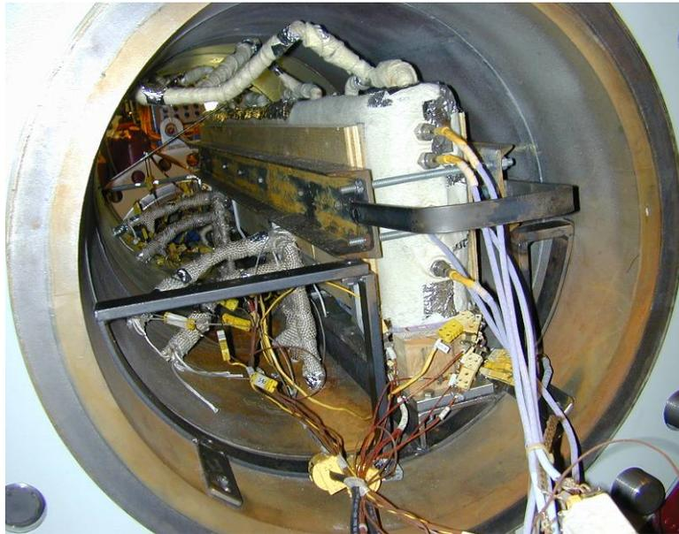
**FIGURE 3-22 TEST MODEL IN THE PRESSURE VESSEL BEFORE THE VESSEL WAS BOLTED AND CLOSED**
