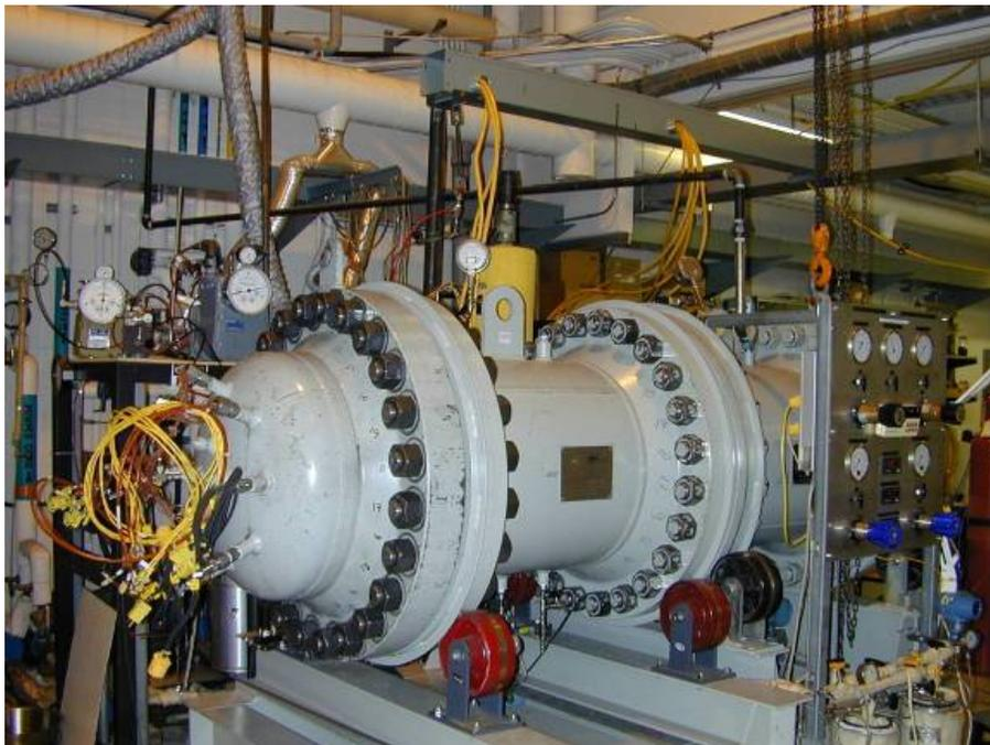
**FIGURE 3-11 TEST FACILITY: COMBINATION OF TWO PRESSURE VESSELS**
