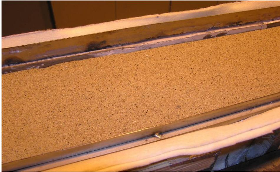
**FIGURE 3-19 TEST CELL PACKED WITH US SILICA SAND: – 20 TO +40 MESH FRACTIONS**
