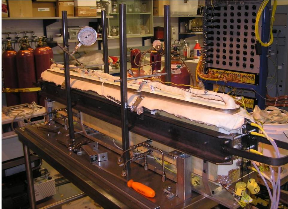
**FIGURE 3-20 LEAKAGE TEST ON THE TEST CELL PACKED WITH SANDS**
