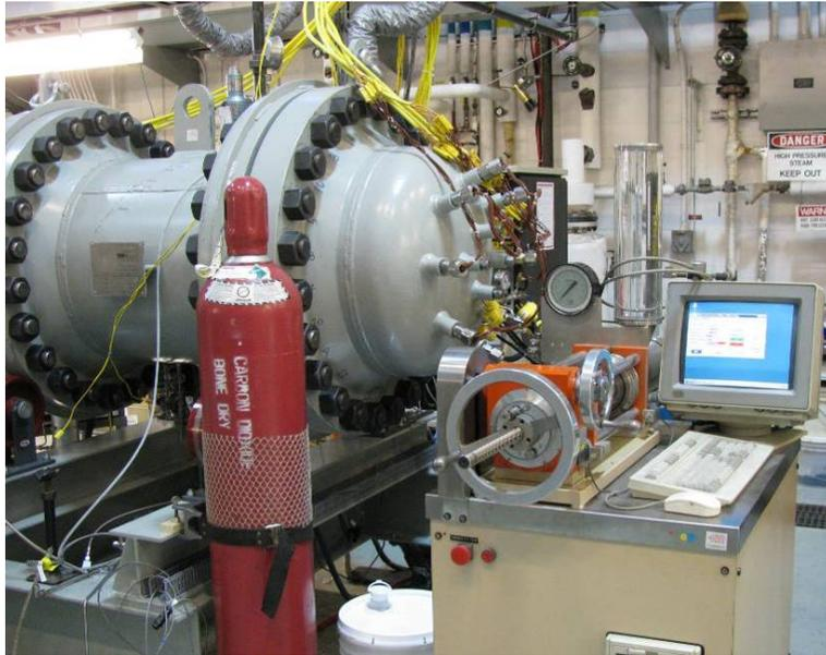
**FIGURE 3-23 EXPERIMENTAL FACILITY: WATER SATURATION BY INJECTING WATER WITH A DBR CYLINDRICAL PISTON PUMP**
