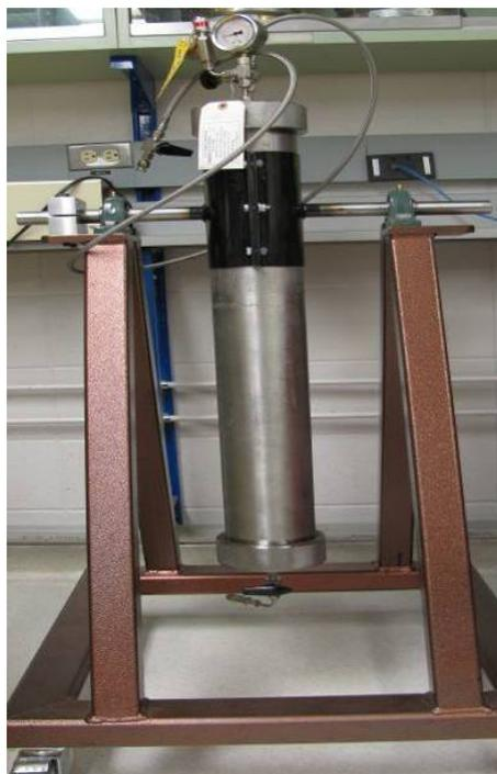
**FIGURE 3-27 ONE 5-L STEEL CYLINDRICAL CONTAINER WITH A PISTON ISOLATING LIVE OIL AND WATER**
