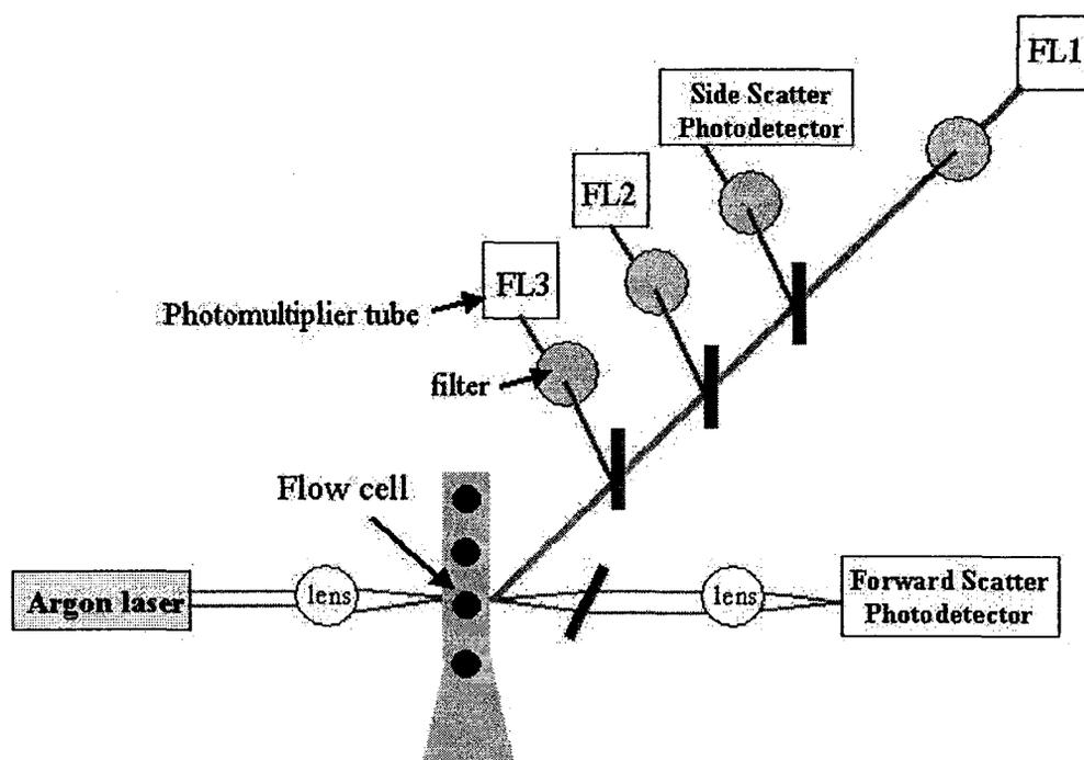
**Figure 14.** Basic principles of flow cytometry. Flow cytometry involves the study of cells under laminar flow conditions. The cytometer is equipped with a 488 nm wavelength argon laser, and 525 nm and 575 nm band pass filters are used for detecting FITC- and PE-fluorescence (FL1 and FL2).
