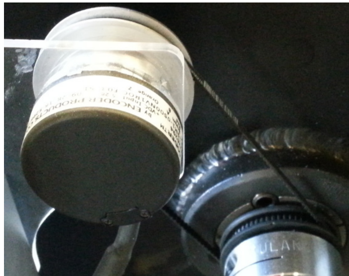
Figure 2.25: Image of the Angular Position Measurement Set-Up
