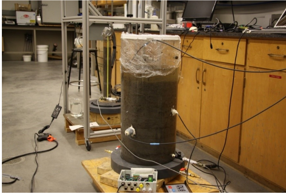
Figure 4. 7 Meso-scale column apparatus using applied suction.
