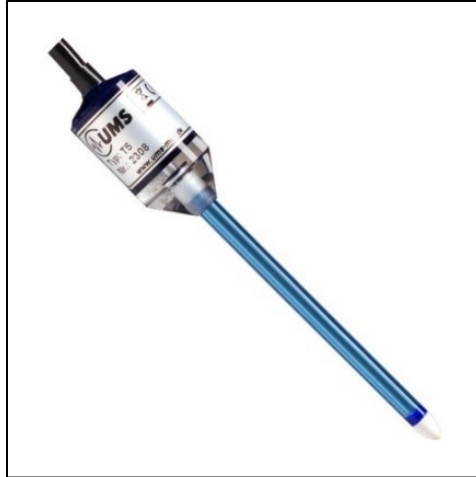
Figure 4. 19 T5 - Negative pore pressure measuring sensor from meter©.
