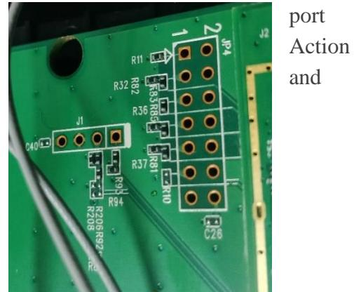
To get access to the console port, a JST connector was needed, and then a USB to Serial (RS232) adapter could be used.
