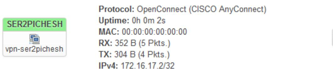
To test the project targets, I checked and made sure that in the first step I can ping my default gateway, while I am connected wirelessly from a laptop to the router. I needed to also check to see if the VPN server is pingable, considering that I do not have any PAT setup over the VPN tunnel, and IP addresses shows the same on the other end of the tunnel.
