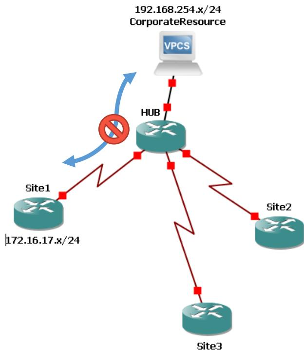
For example, “vpns0” as the new dynamic network interface which is created after the first established connection, needed to have forwarding access to the “ens160” which is the corporate resource.
