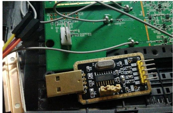
At this step, I needed to find the pinout to determine the VCC/GND/TX and RX. I can easily use a voltmeter to do this job by grounding the voltmeter by antenna connector and connecting the other end to the pins. The VCC was 3.4, the TX was at a voltage around 3 volts, and the RX and Ground were at 0 volts.
