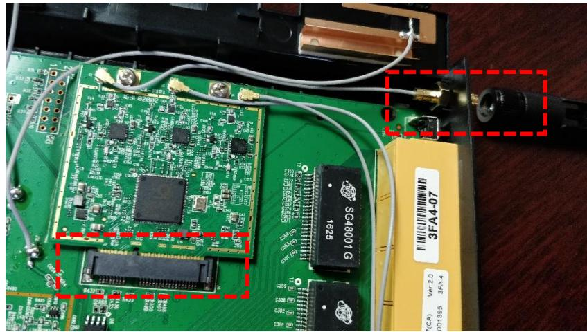
In contrast, version 4 to 5 are equipped with three dual 2.4 and 5GHz antennas.
